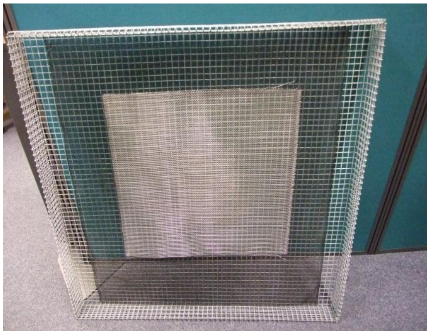
Figure 16: Picture of the trays that were designed for the herbicide testing. The outside trays coming in direct contact with herbicides wash off covered with stainless steel while trays were lined with coated aluminum material.
