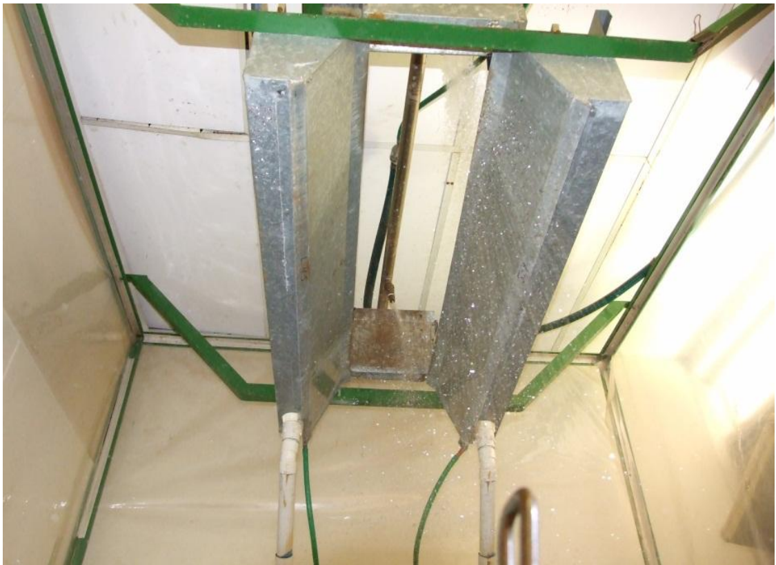
Figure 12. The oscillating boom rainfall simulator used for the testing. The pictures shows the two nozzles as they oscillate from one side to another
