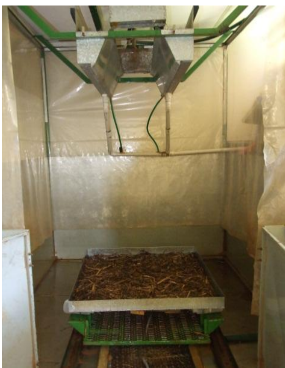
Figure 15. Rainfall Simulator with a tray of trash placed underneath ready for rain.
