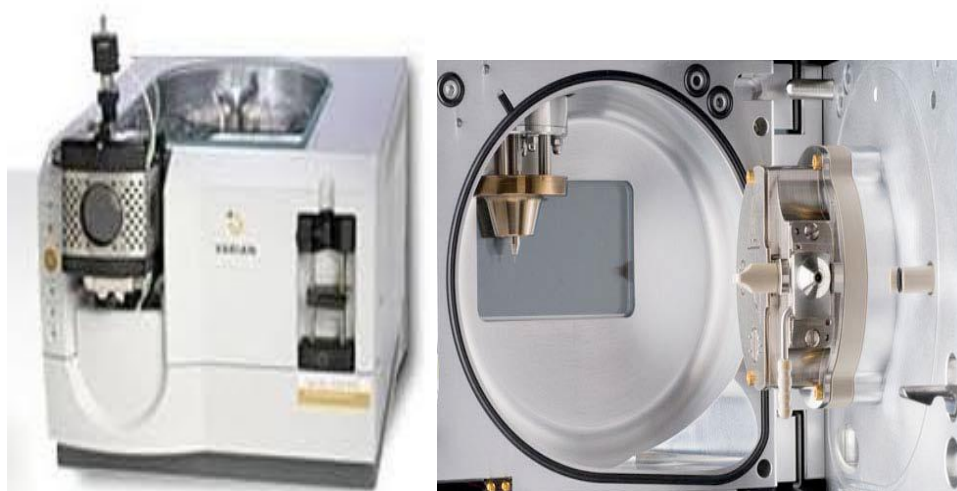
Figure 18. The combination of a mass spectrometer and a high performance liquid chromatographer.
