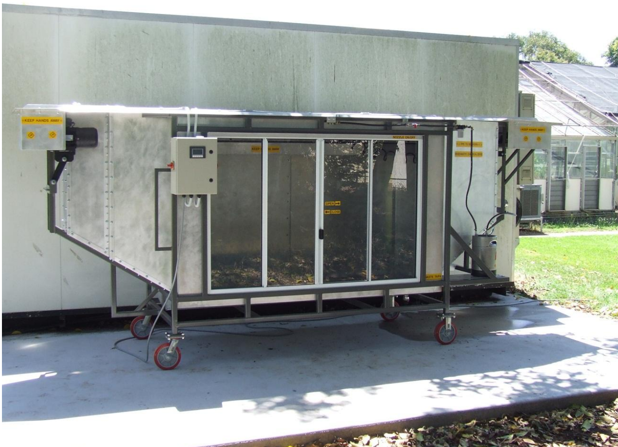
Figure 11. Leslies Research Centre's Spray cabinet that was used to uniformly spray the herbicides on the trash trays. This sprayer ensures that each tray received the same amount of each herbicide at the same rate.
