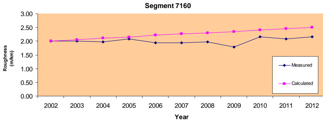
Figure 5.33 Comparison of predicted versus actual roughness for Segment 7160 at Elsmore
