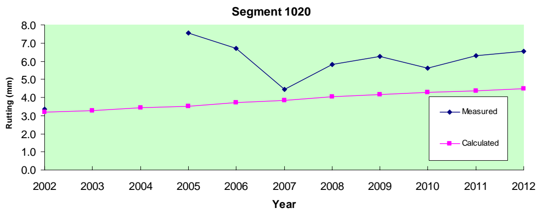
Figure 5.31 Comparison of predicted versus actual rut depth for Segment 1020 at Waterview
