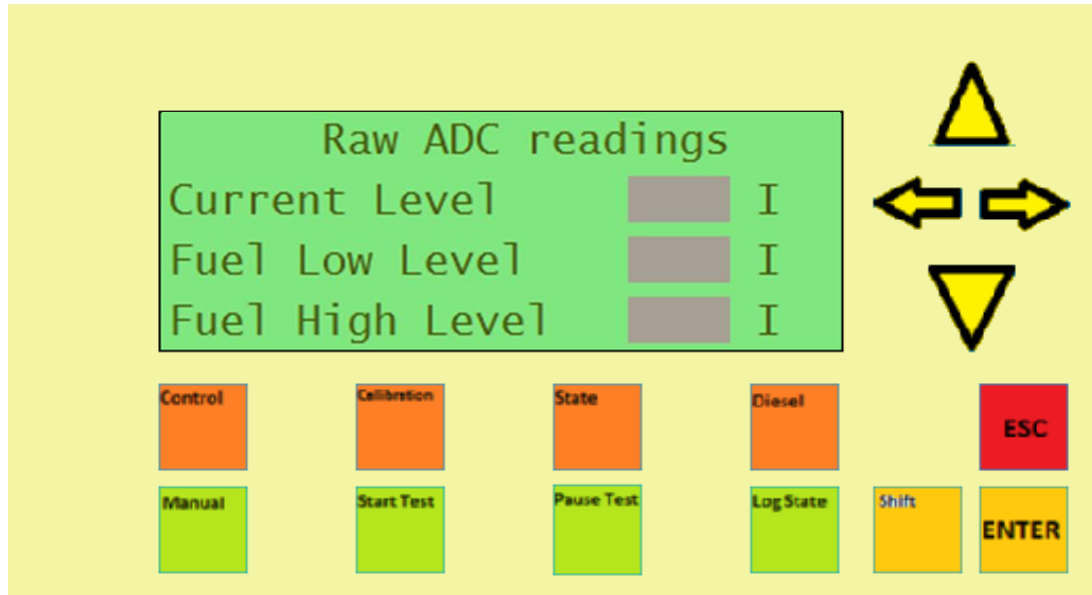
Figure 15: Text display of ultrasonic level sensor real time level and limits.
