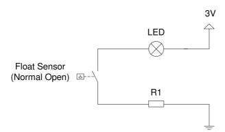
Fig 4.13 Drawing of the initial circuit design
