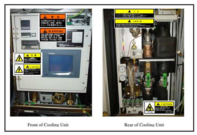
Fig 6.5 Location of warning labels in the cooling unit
