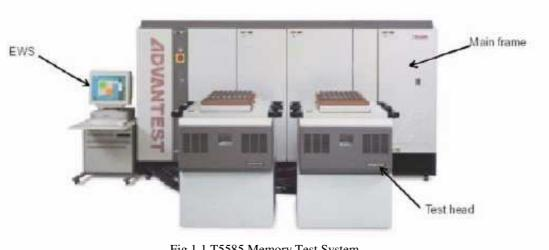
Fig 1.1 T5585 Memory Test System
