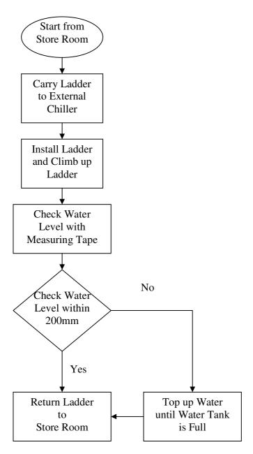
Fig 2.3 Water Level Monitoring Flow Chart
