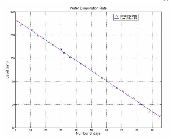
Fig 3.7 Plot of Water Level (mm) versus Number of days
