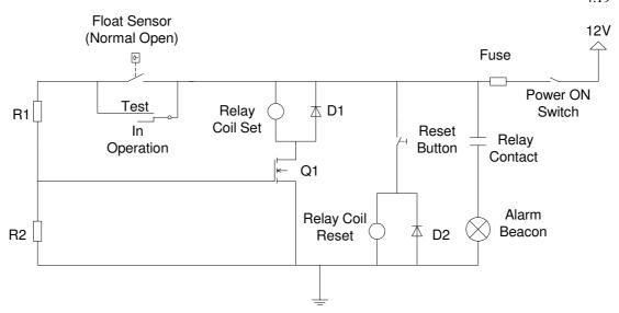
Fig 4.14 Normally Open Float Sensor Circuit Design
