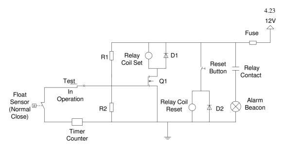
Fig 4.16 Timer counter added into the normally close circuit
