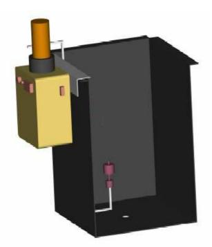
Fig 4.23 Water level detection jig attached to water tank
