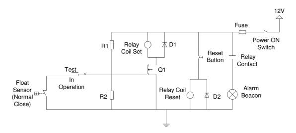
Fig 4.15 Normally Close Float Sensor Circuit Design
