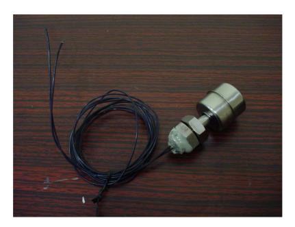
Fig 4.10 Vertical Float Sensor
