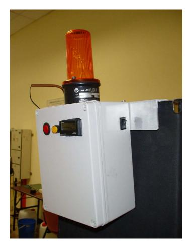
Fig 4.24 Water level detection jig attached to the water tank
