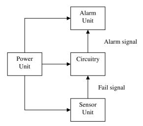
Fig. 4.6 Simplified Block Diagram of the Water Level Detection Jig
