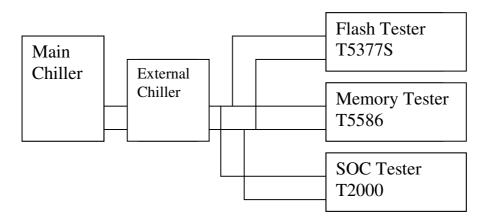
Fig 1.5 Layout of the Test Floor
