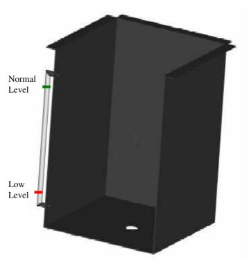
Fig. 4.3 Visual water level monitoring tube
