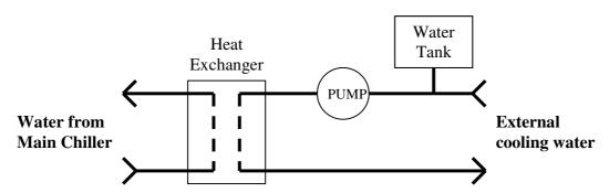
Fig 1.7 Simplified Block Diagram of the External Chiller
