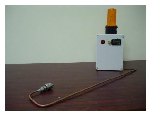
Fig 4.22 Water level detection jig
