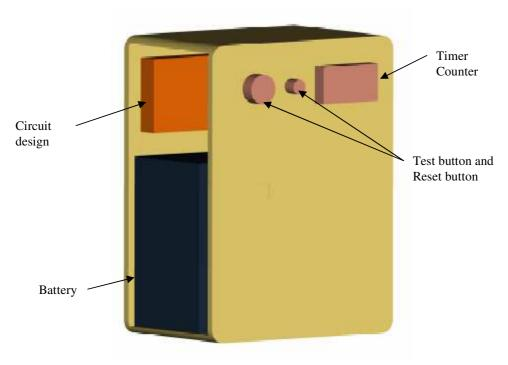
Fig 4.19 Control Box layout
