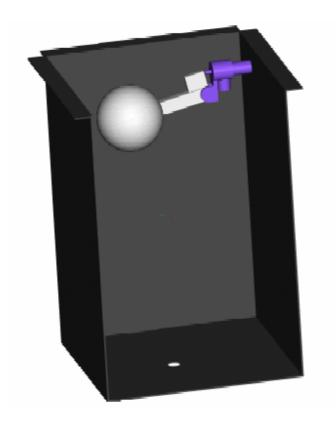
Fig. 4.1 Toilet Flush System attached to the water tank
