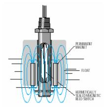
Fig 4.8 Drawing of a typical Vertical Float Sensor (Source: The Control Components Australia 2003)
