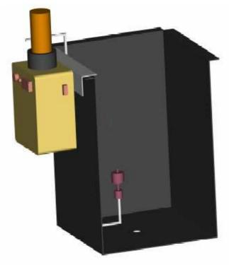
Fig 4.4 Water Level Detection Jig
