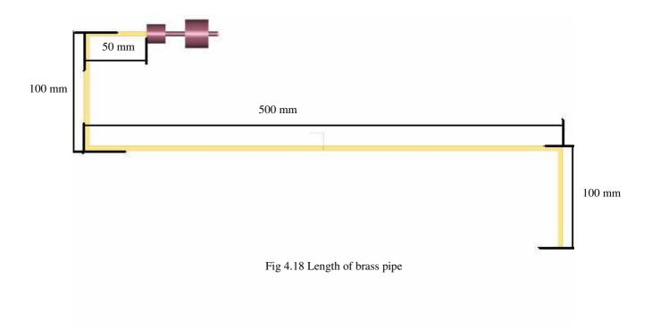
The height of the water tank is 460 mm. Therefore a longer mid section is required. Figure 4.18 shows the length of the brass pipe that is required. The total length of the brass pipe required is 750 mm.
