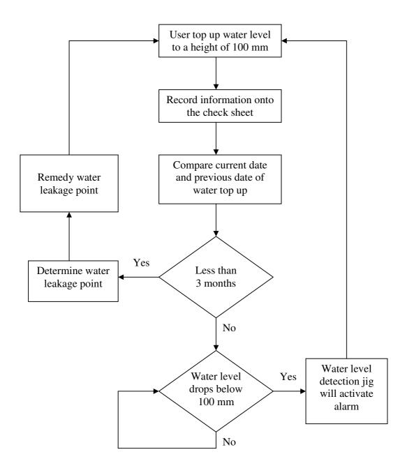
Fig 5.2 Flowchart of the water leakage detection sequence
