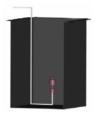
Fig 4.17 Float sensor placed vertically in the water tank
