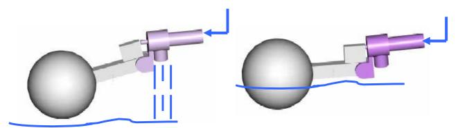
Fig. 4.2 Float position at different water level height
