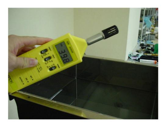
Fig 3.3 Relative Humidity surrounding the External Chiller
