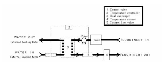
Fig 1.2 Simplified Block Diagram of the Cooling Unit
