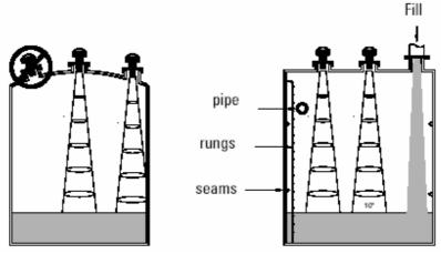
Fig 4.9 Location of the Ultrasonic Sensor (Source: The Siemens Process Instrumentation 2006)
