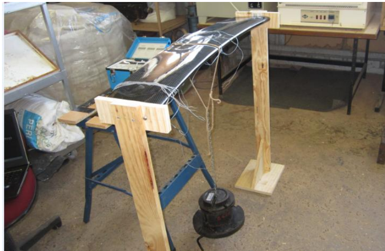
Figure 5.4 – The Strain Testing Assembly
