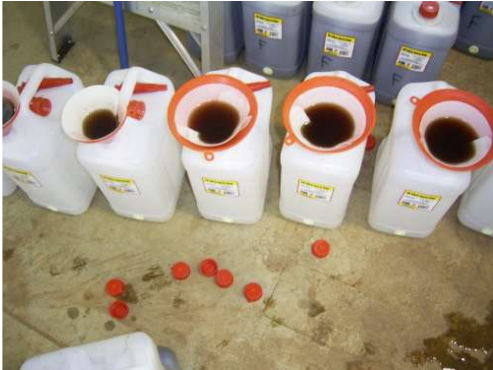
Figure 3.1: Secondary filtration process using 3 um pore size, Whatman filter paper for fine particle retention
