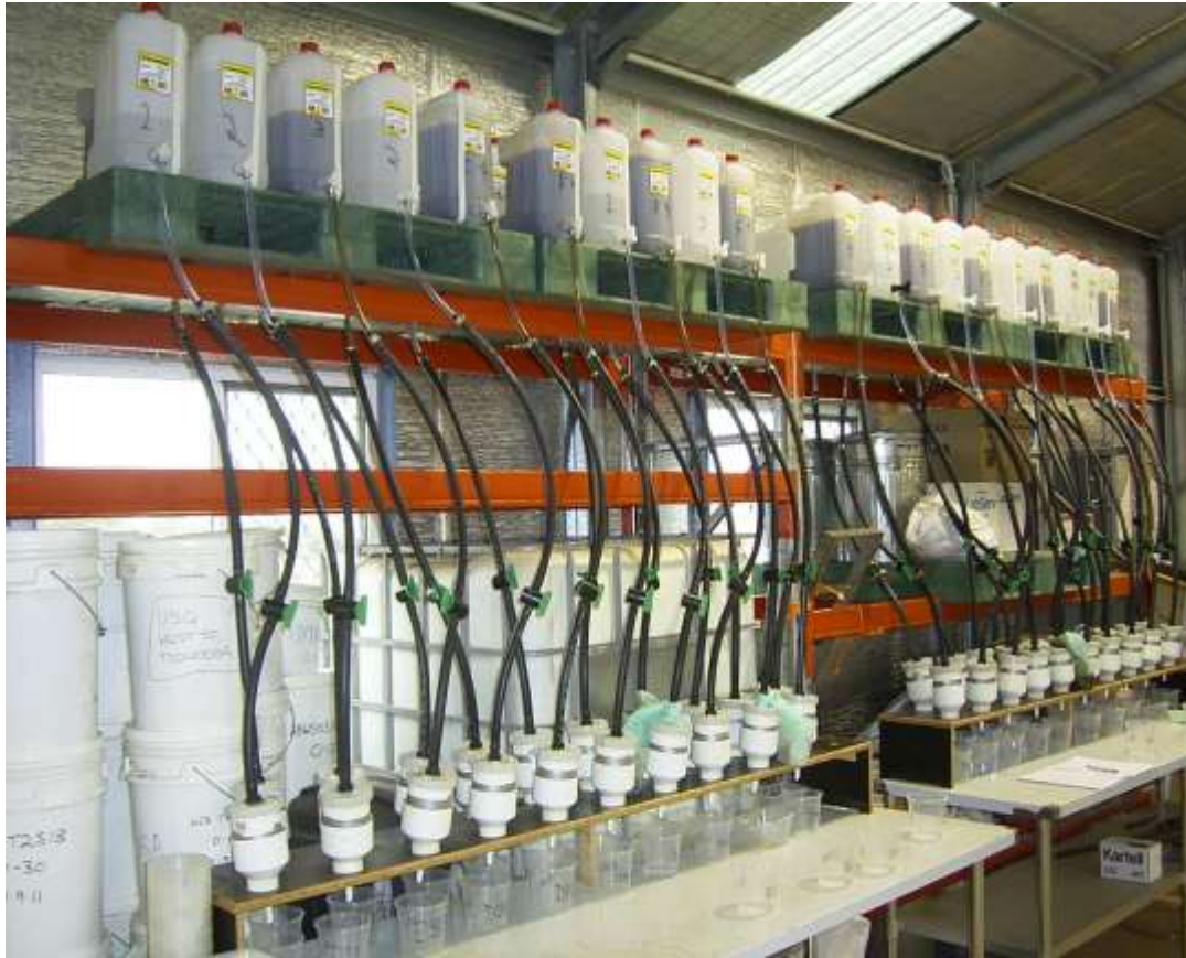
Figure 3.5: Fully constructed apparatus for measuring HC via falling pressure head
