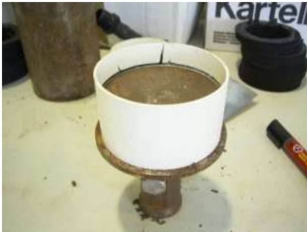
Figure 3.2: Soil Core Compaction depth measurement for 98% MDD
