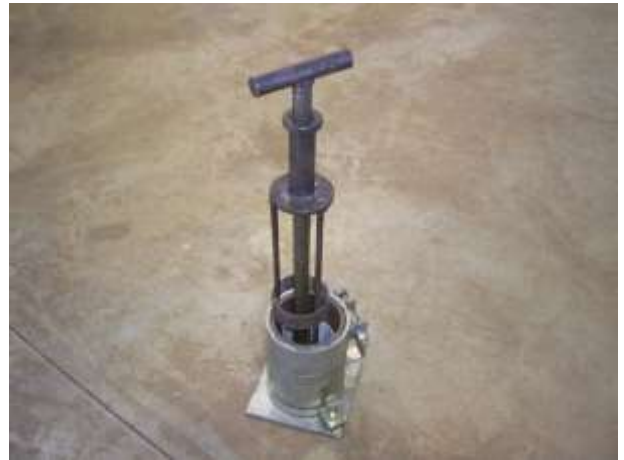
Figure 3.3: Quick release compaction cylinder and standard hammer used in soil compaction process
