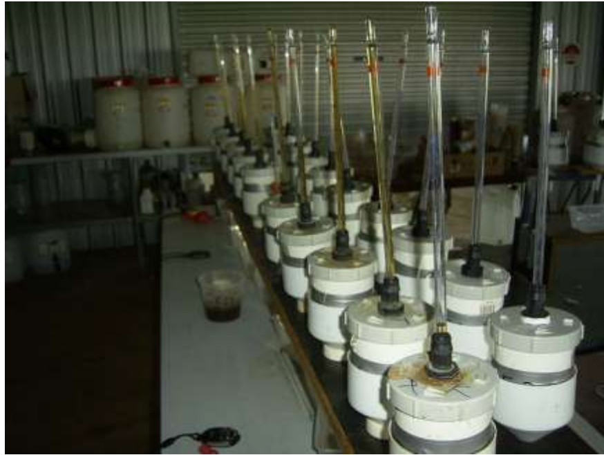
Figure 3.6: Pipette analysis to obtain the final HC reading
