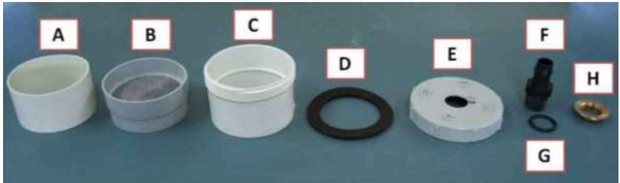
Figure 3.4: Soil Core Construction: A) soil core, B) 90 mm mesh filter socket, C) 90mm coupling, D) 3 mm thick neoprene gasket, E) screw-on end cap, F) 19mm nozzle, G) o-ring, H) brass nut
