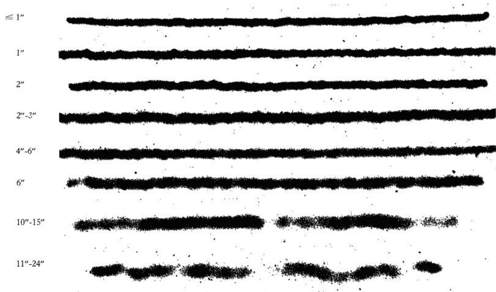
Figure 3.2: Star trails of Polaris with estimates of the Stellar Image Diameter using the 120-inch Telescope (adapted from Harlan & Walker (1965)).
