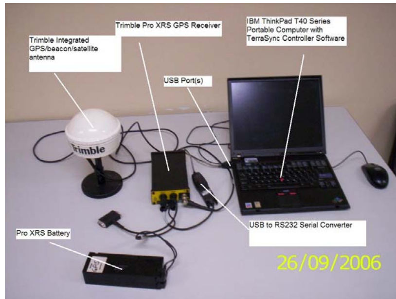
Figure 3.2: Static Test Equipment
