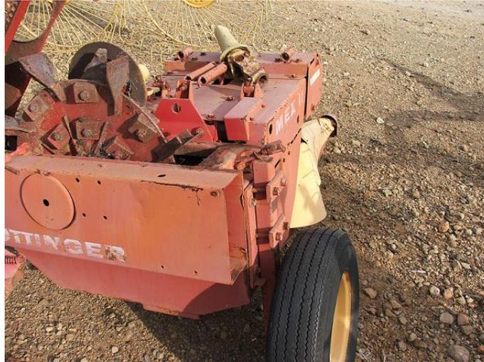
Figure 3.4: Disc chopper configuration where material is chopped and ejected with the same disc (Personal Photo).
