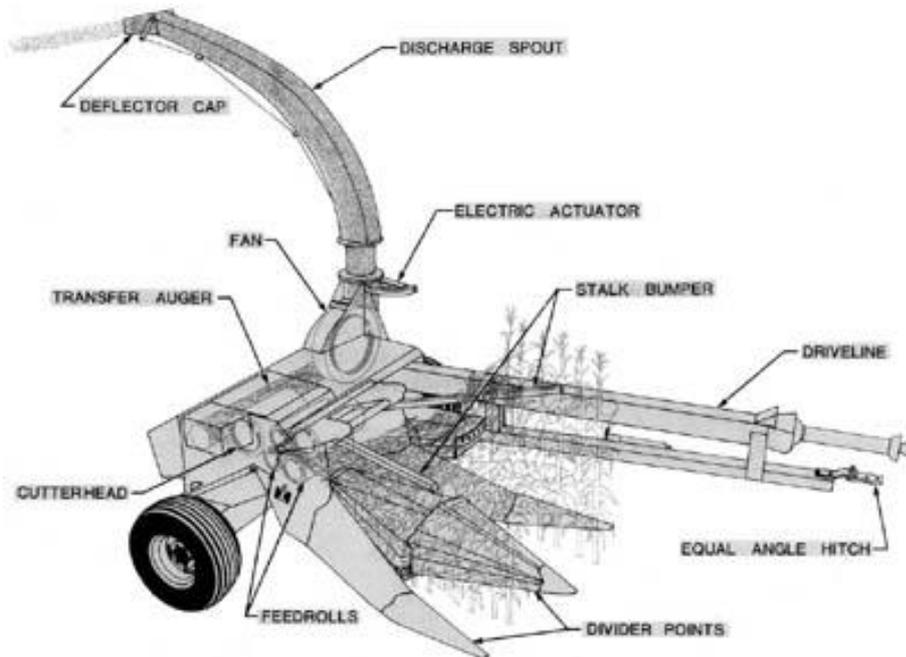
Figure 3.6: Cut and blow design (Slingerland 2003).
