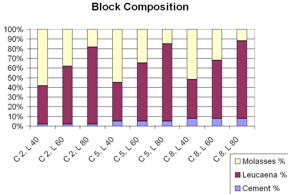
Figure 4.5: Mixture composition of second experiments.
