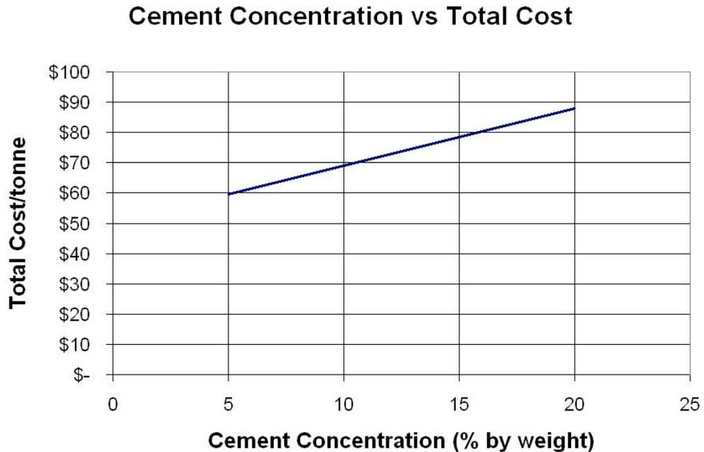
Figure 5.5: Extrapolation of cement ratio vs dry matter achieved.
