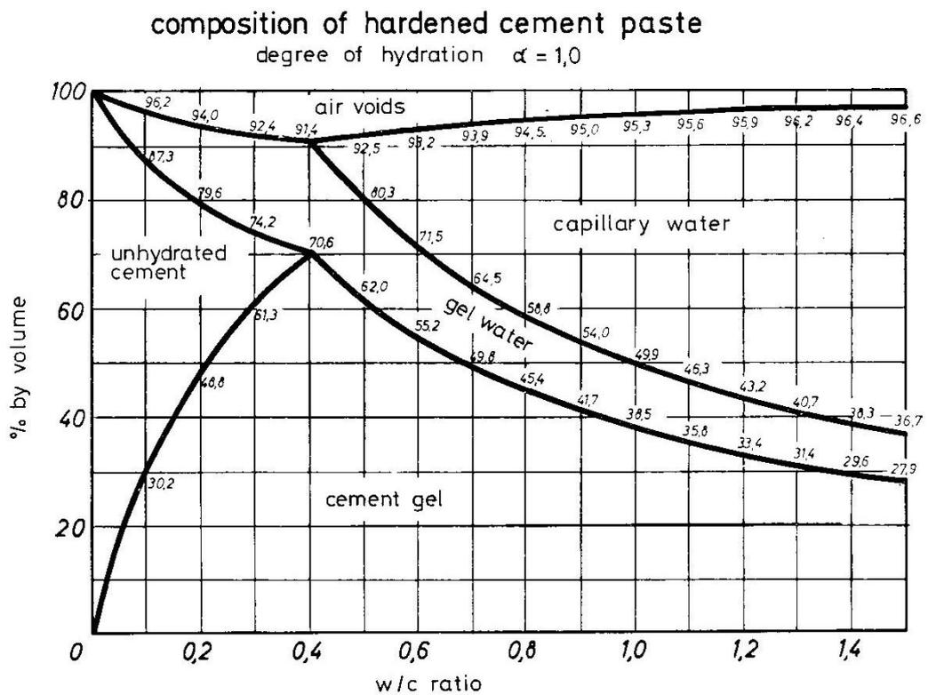
Figure 5.3: Parts by volume of the respective components of hardened cement past as a function of water/cement ratio, 100% hydration (Czernin 1980, 63).
