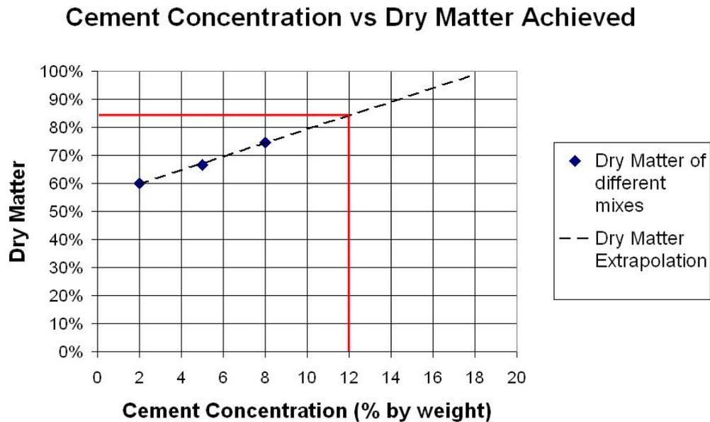
Figure 5.4: Extrapolation of cement ratio vs dry matter achieved.
