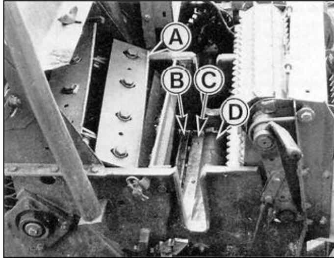
Figure 3.3: Drum chopper assembly showing (A) Rotating Knives, (B) Shear Plate, (C) Scraper, (D) Smooth Feedroll. Material flows from right to left (Ragan 2002).
