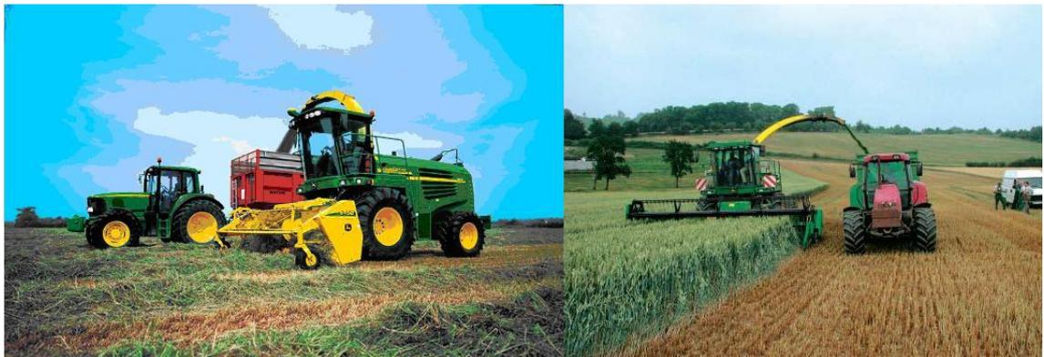
Figure 3.5: John Deere forage harvester with pick-up front (left) and header front (right) (*John Deere Self-Propelled Forage Harvester Web Brochures 2006*).
