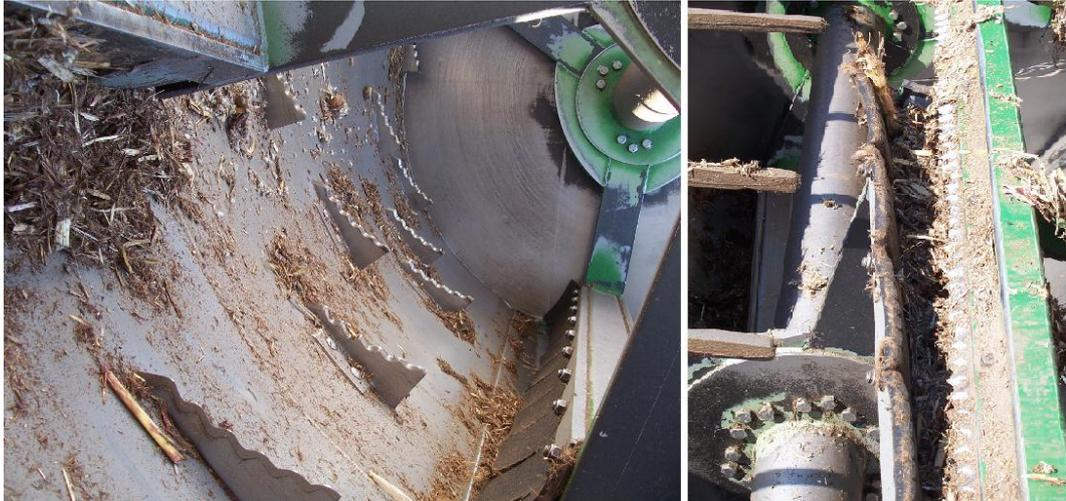
Figure 5.2: Picture of Killara's feed mixture showing knife arrangements (Personal Photo).
