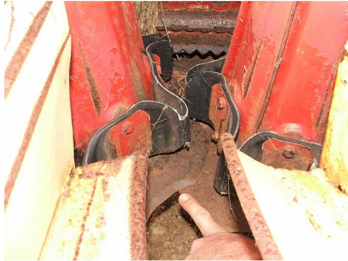
Figure 3.10: Cutting action of POTTINGER harvester (Personal Photo).
