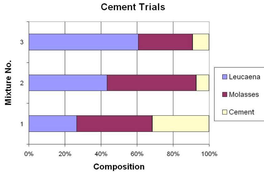
Figure 3.1: Mixture composition of cement-based blocks.
