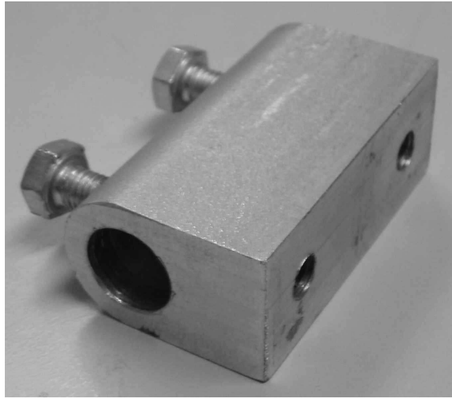
Figure 2.7: Connector component of the Modular Robot's mechanical structure.
