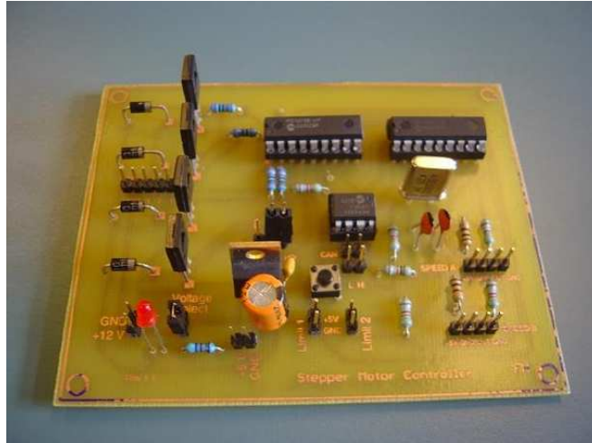
Figure 3.2: Stepper motor control module.
