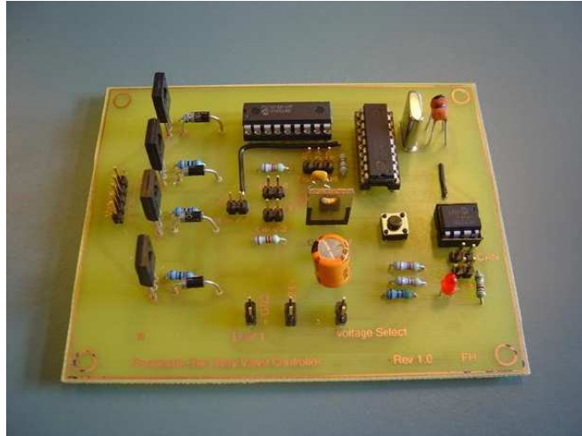
Figure 3.4: Pneumatic two-way valve controller.
