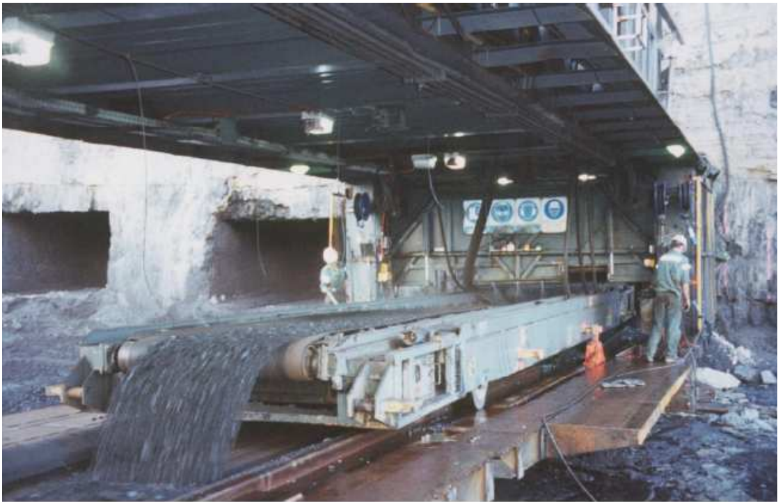
Figure 2-8 Addcar Steep Dip Highwall Mining Machine at Moura Mine (Shen & Duncan Fama 2001)
