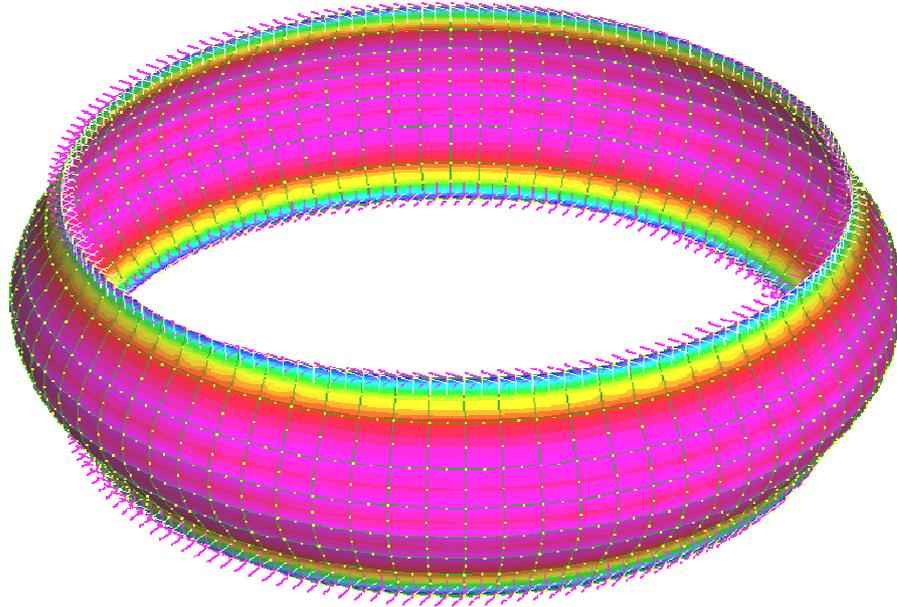
**Figure 4.2: Contour plot of stress distribution (YY axis).**
