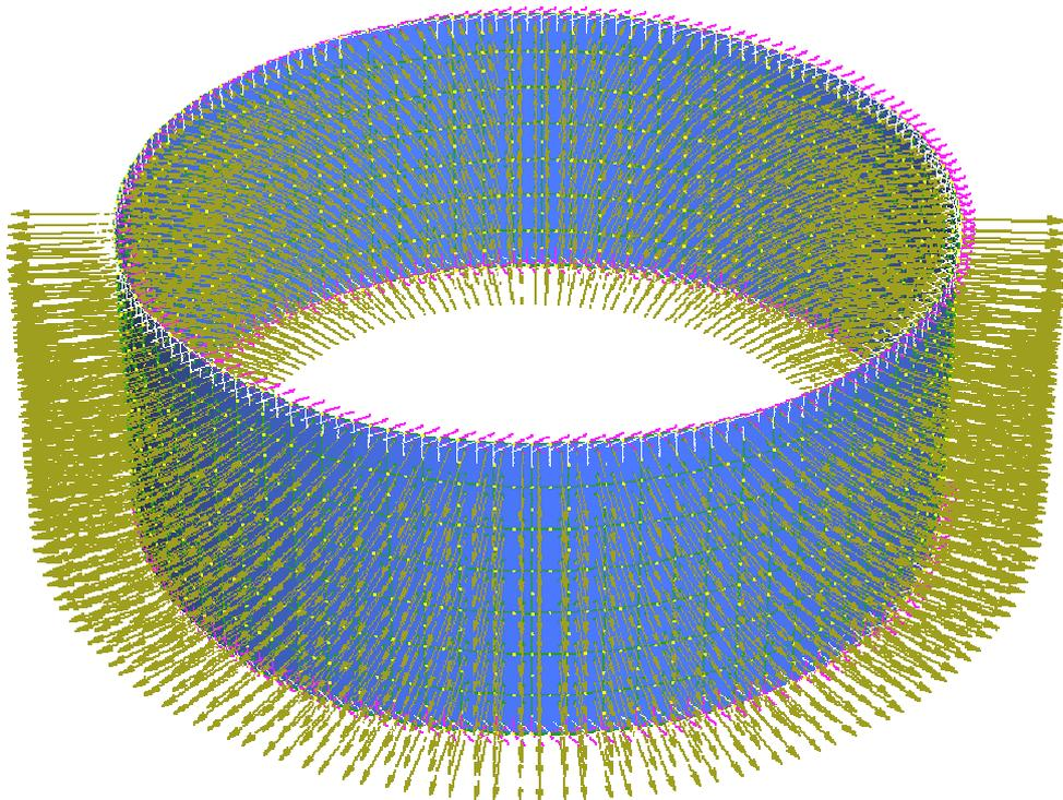
**Figure 3.3: Finite element model subjected to lateral face pressure.**
