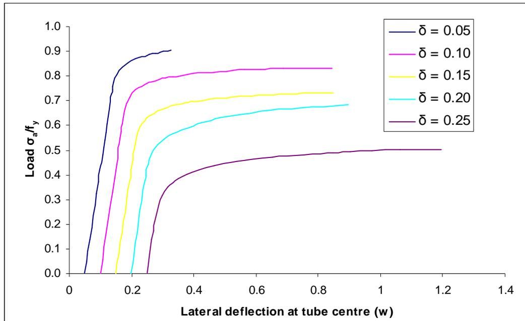
Figure 5.3: Load-deflection curves for tubes with different geometric imperfections.
