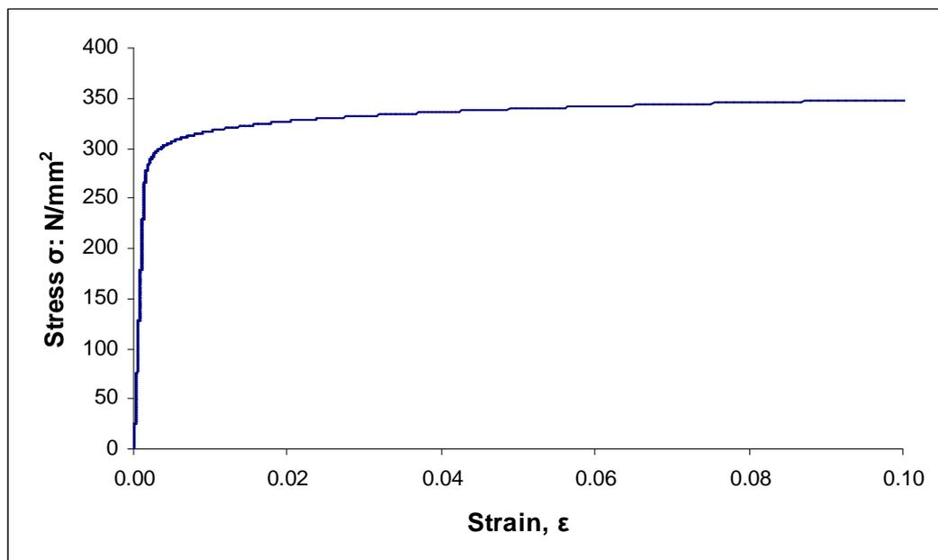
Figure 3.5: Stress-strain curve based on the Ramberg-Osgood model.
