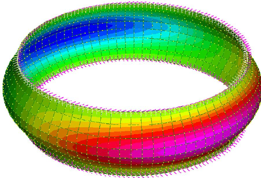
**Figure 4.1: Contour plot of displacement (DX axis).**
