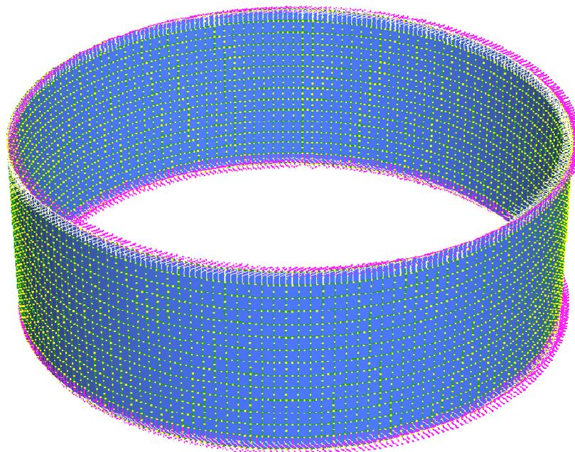
**Figure 3.2: Finite element model with a mesh size of 12x12 mm.**
