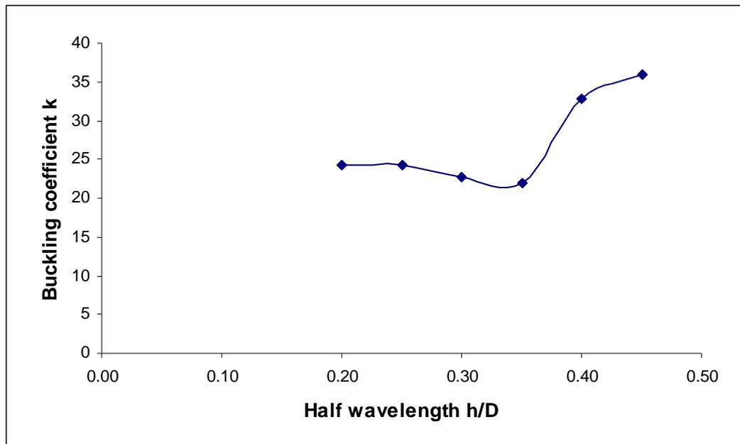
Figure 5.2: Buckling coefficient versus half wavelength.
