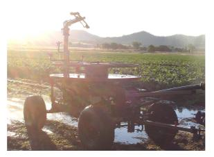
Figure 2.3: Trolley-winch irrigator after use
