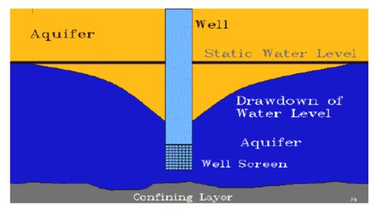
Figure 2.1: Pumping from an underground aquifer
