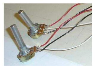
Figure 5.1: Potentiometers used in prototype
