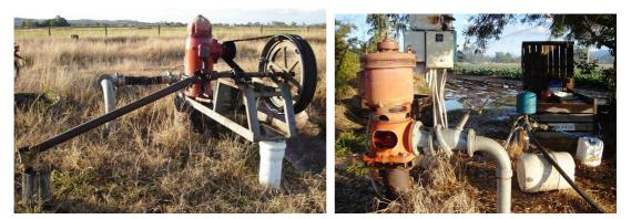
Figure 2.2: PTO driven (left) and electrically powered (right) irrigation pump
