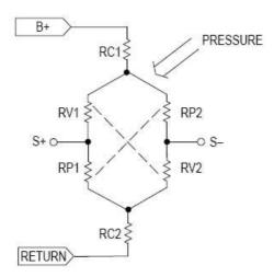
Figure 2.4: Pressure Sensor Circuit (*Warren Shultz, Motorola Inc., 1997*)
