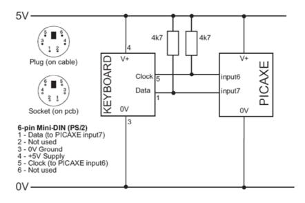
Figure 3.2: Wiring used to connect keyboard to PICAXE 18X (Image from PICAXE Manual 2, Revolution Education, p40, 2004)
