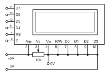
Figure 3.1: Connections for LCD module to PICAXE 18X (*Image from PICAXE Manual 3, Revolution Education, p34, 2004*)
