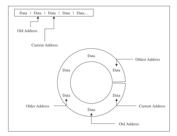
Figure 4.3: Graphical representation of data overwrite structure
