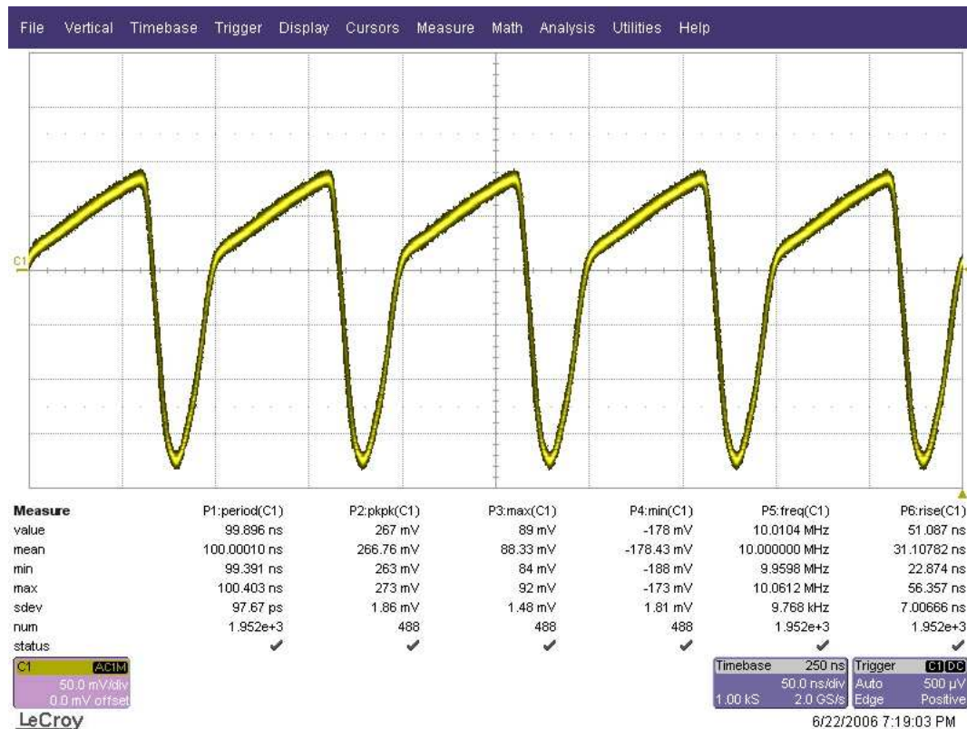
Figure 30: Test Point T1 Output Waveform using LeCroy Wave Surfer 424
