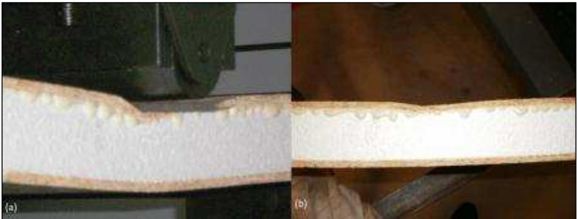
Figure 4.16: OSB panel failing
