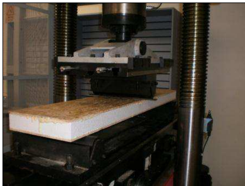
Figure 4.13: OSB panel positioned in the bending machine
