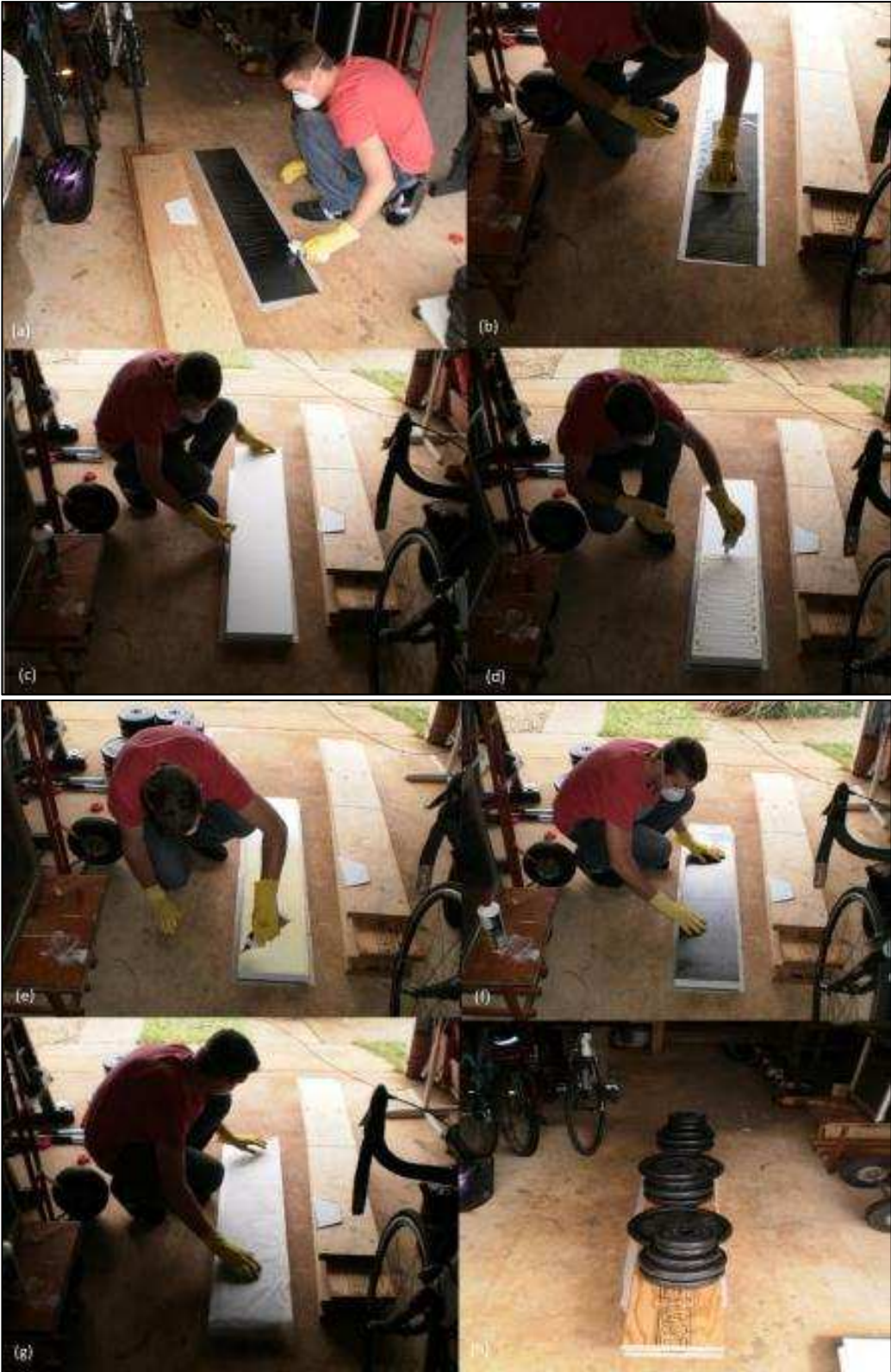
Figure 4.9: Assembling an EPS core panel
