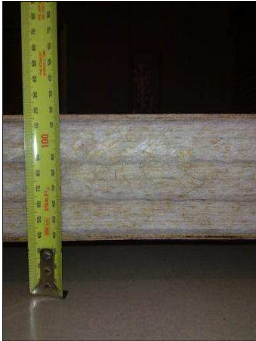
Figure 4.22: Measuring the BFC Panel prior to loading
