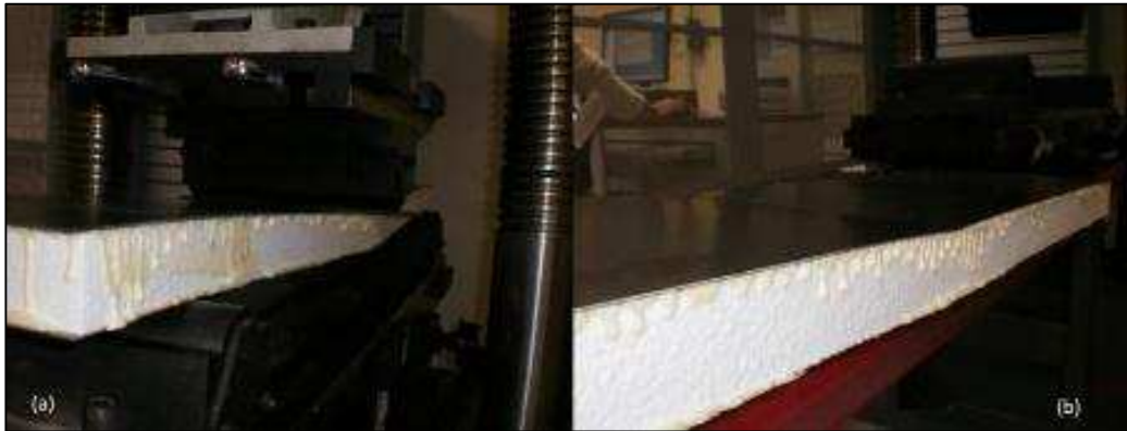
Figure 4.20: Steel Panel Failing
