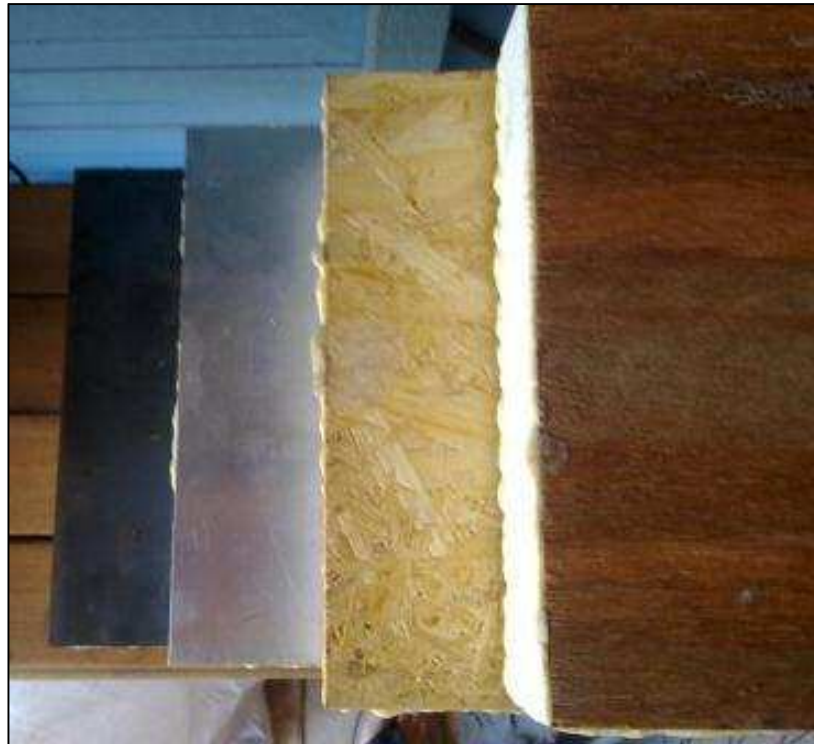
Figure 3.1: Face Materials – Steel, Aluminium, OSB and Plywood
