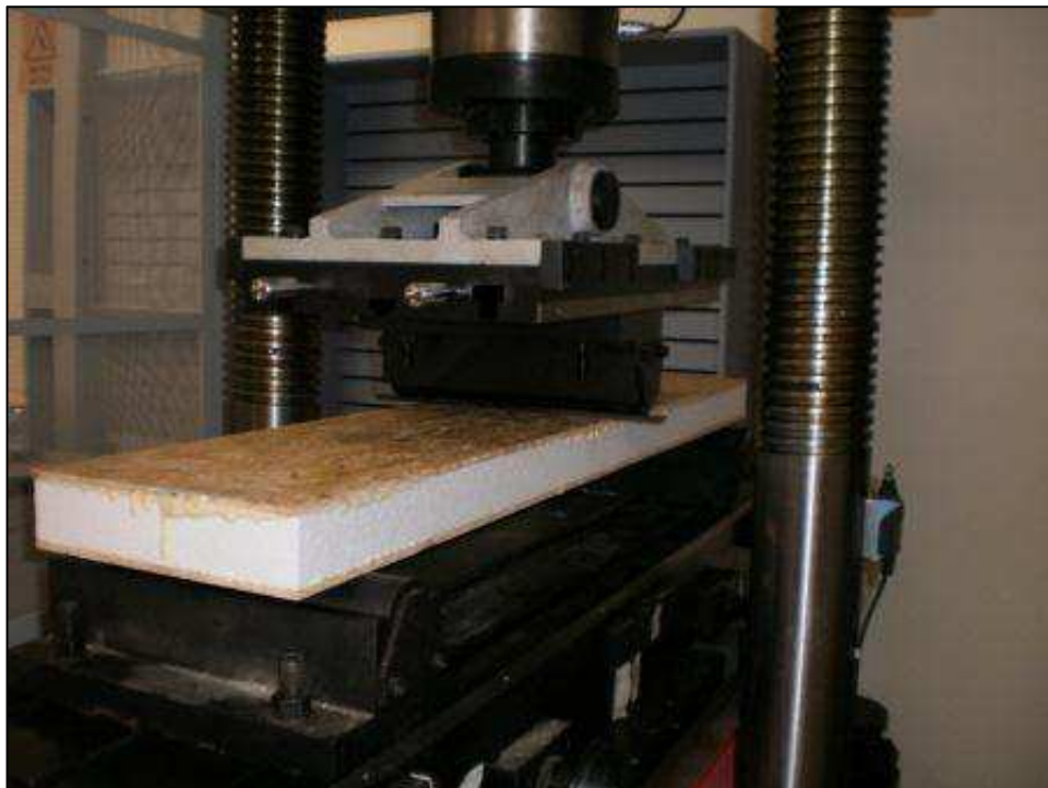
Figure 3.6: OSB Faced Sandwich Panel under 3-point Bending
