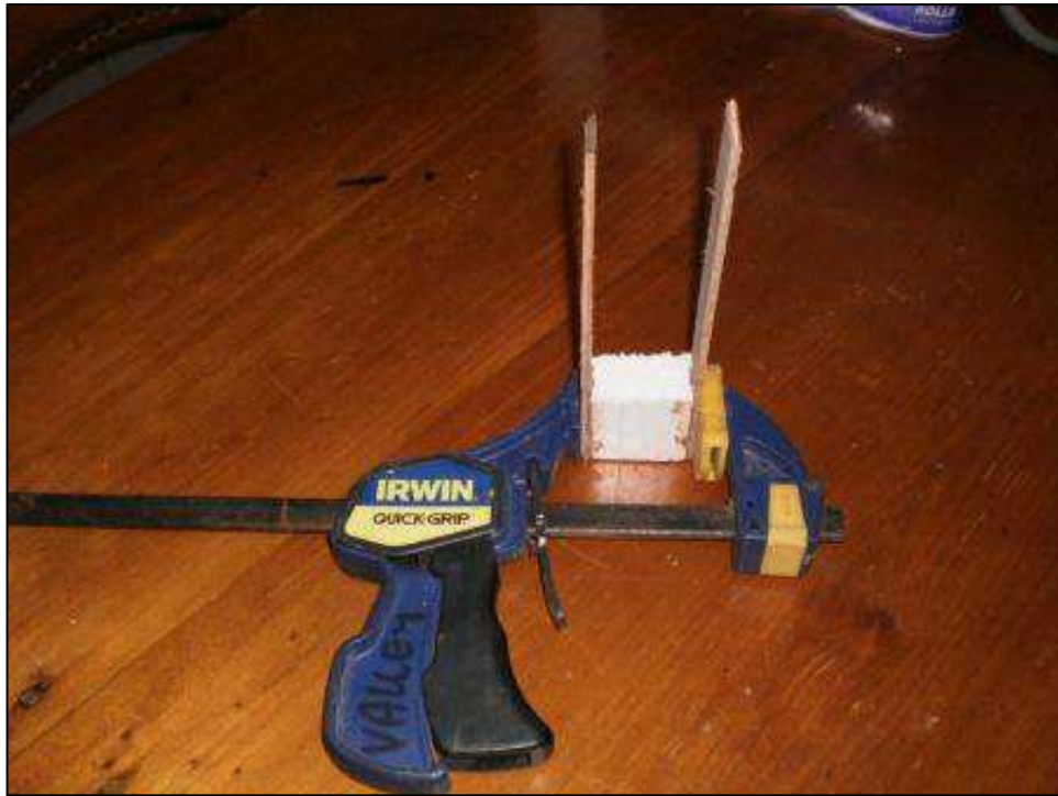
Figure 4.2: Clamping adhesive test rigs to allow glue to set.
