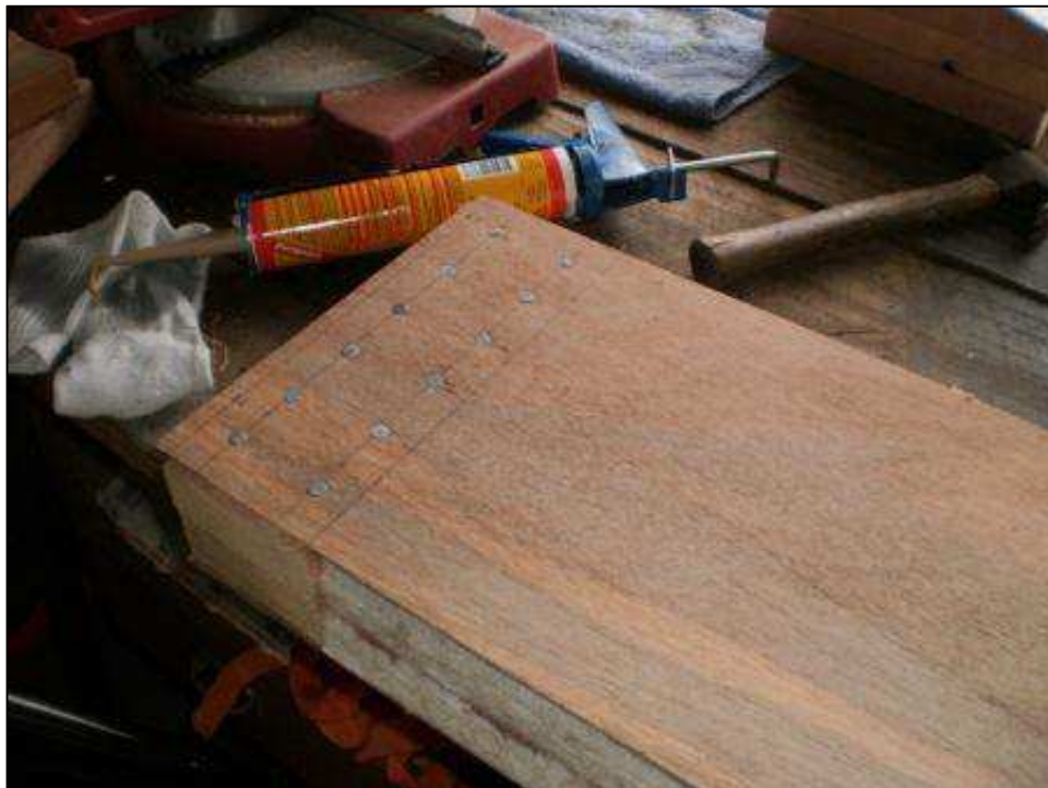
Figure 4.11: BFC core panel with timber bearing block
