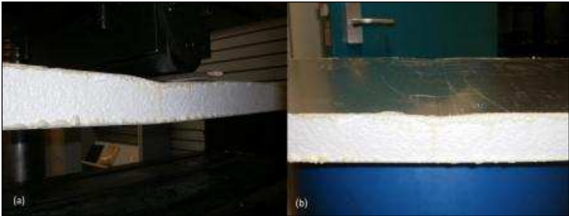
Figure 4.18: Aluminium panel failing
