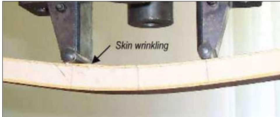
Figure 2.3: Face Wrinkling Under Four Point Bending (Manalo et al. 2010)
