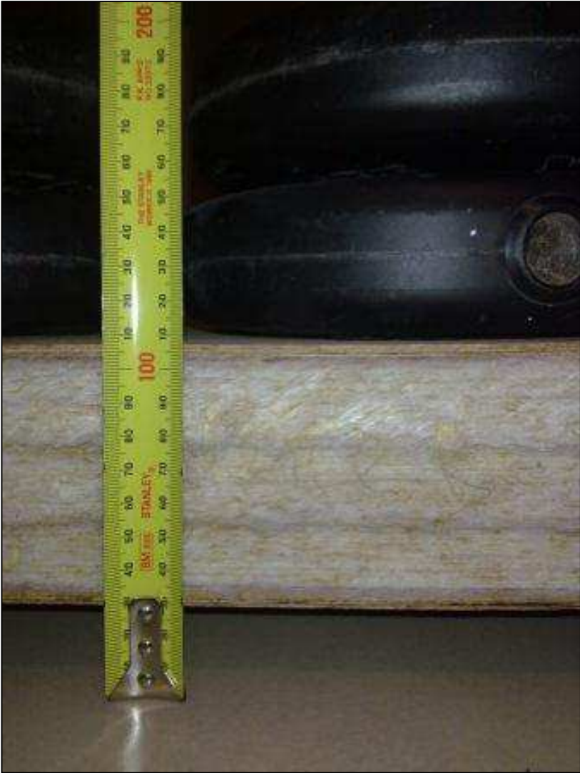
Figure 4.23: BFC Panel deflecting under load
