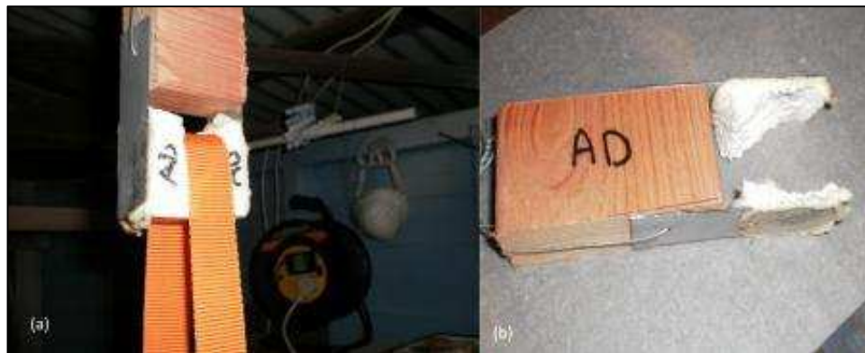
Figure 4.5: (a) EPS compressing and tearing, (b) EPS failure
