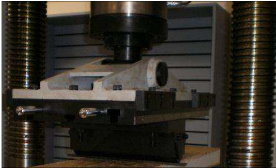
Figure 5.4: SANS Machine centre roller and ram
