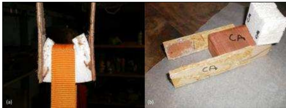
Figure 4.6: (a) CA beginning to fail, (b) Adhesive failure
