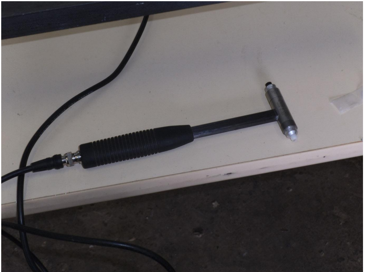
Figure 10 The PCB086C04 impulse hammer which was used to excite the system
