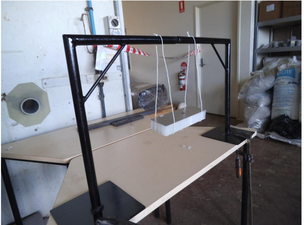
Figure 11 A aluminium skinned sandwich panel suspended in the free-free conditions
