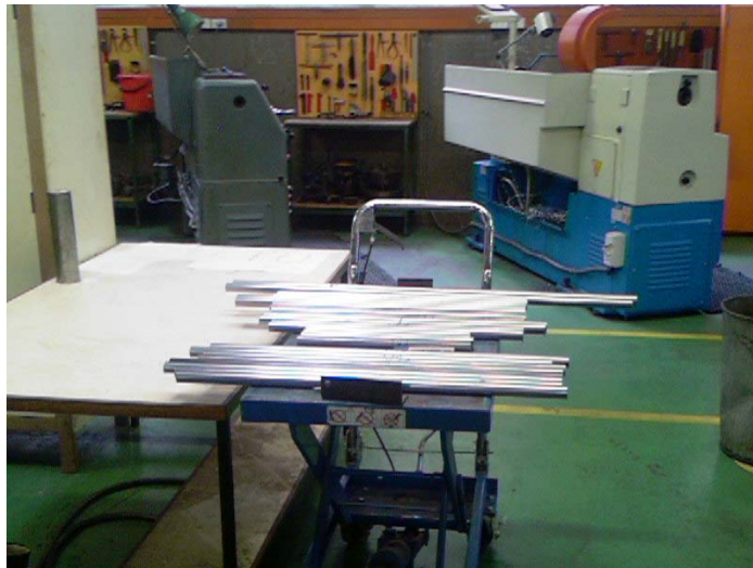
Figure 42: All of the pipes cut to length waiting to be added to the chassis throughout construction.
