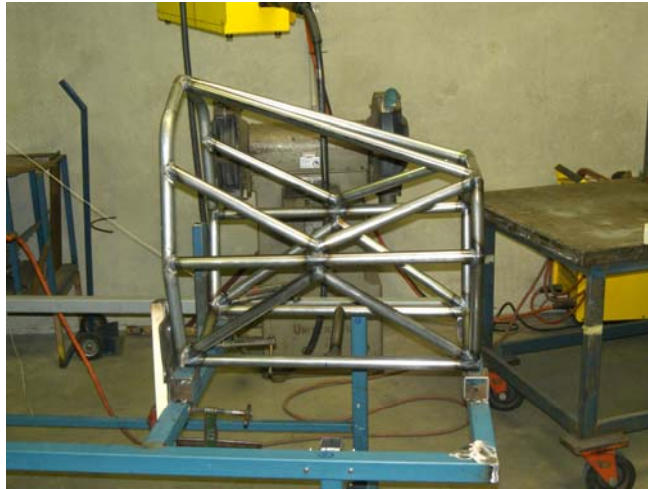
Figure 45: Spider added to the frontal area of the chassis.
