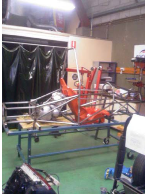
Figure 47: The final design fully constructed with the engine and seat in position to check the design was suitable
