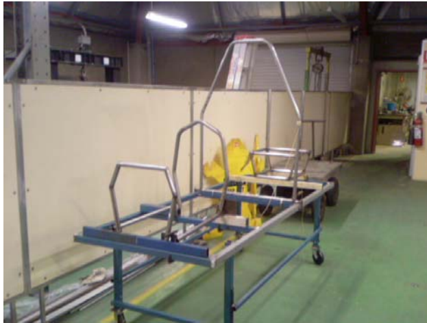
Figure 43: The main components positioned on the construction bed
