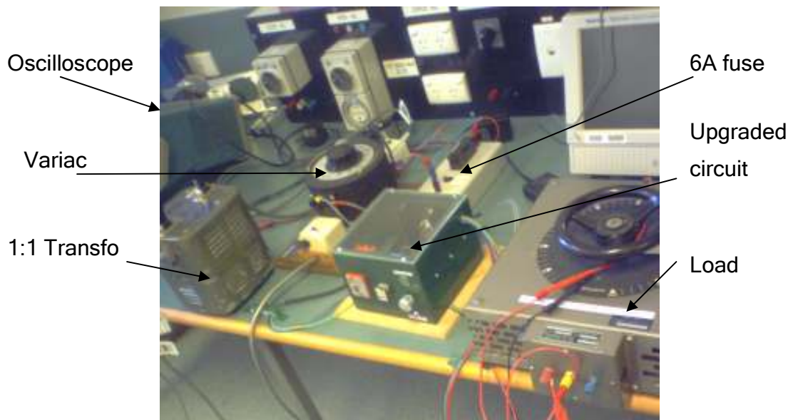
Figure 6.10: Testing configuration of the upgraded system
