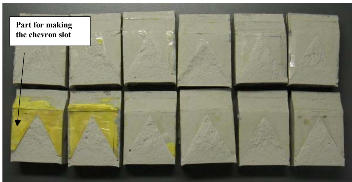
Figure 9.1: The fractured specimens and show the part for making the chevron slot
