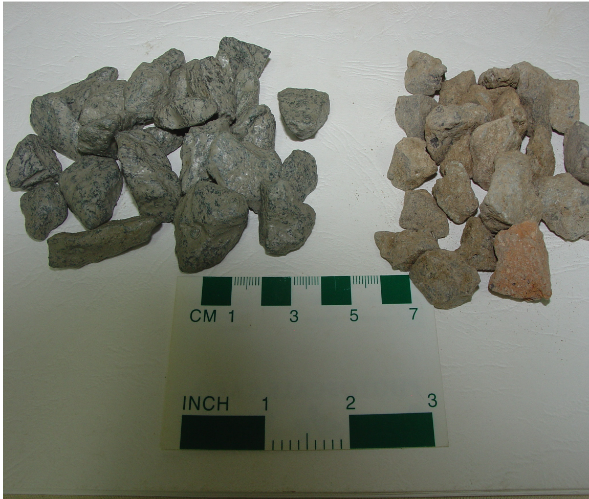
Figure 3.16 Sized 20mm Natural Aggregate (left hand side) and Recycled Aggregate (right hand side)
