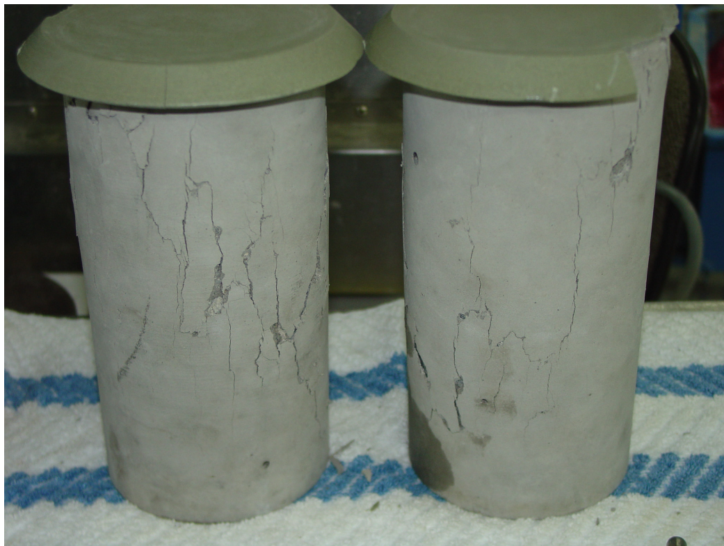
Figure 6.3 7-days Cylinder broken by compressive strength
