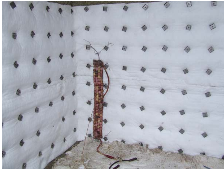
Figure 4.2 a- Furnace wall experiment setup (without covering insulation)
