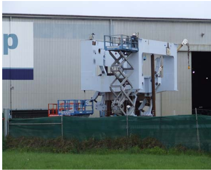
Figure 1.2- Iron Ore Car Dumper Body after stress relief and coating
