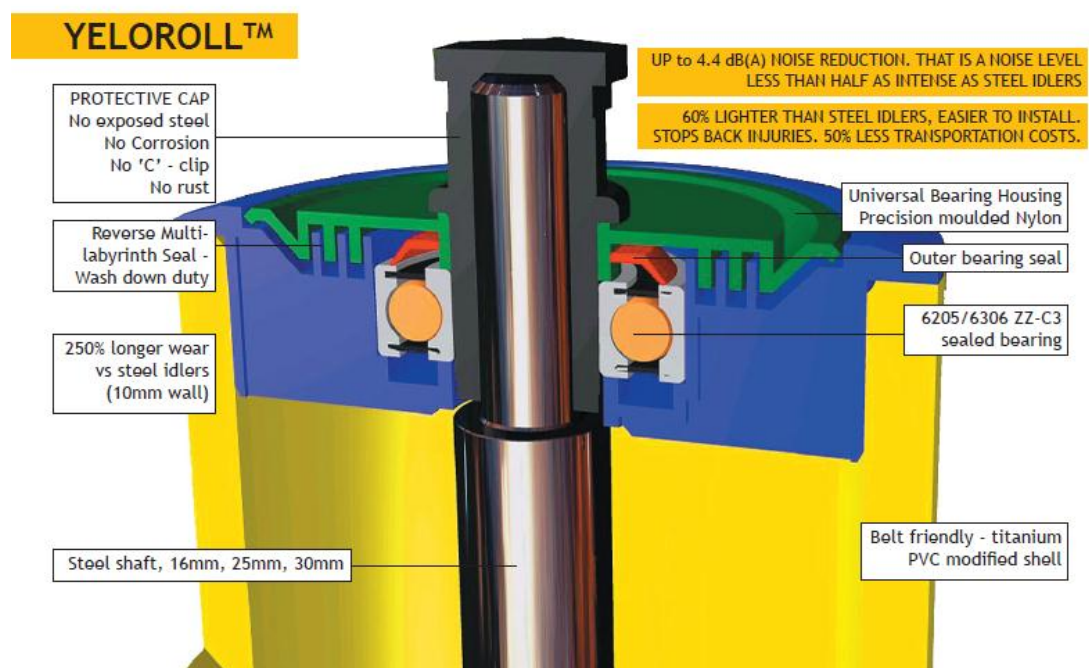
Figure 2-21: Yeloroll idler half roller cut away (Yeloroll 2012)
