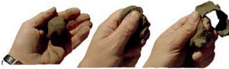
FIGURE 2.8 - STEPS FOR TESTING THE SOIL BOLUS (WWW.VRO.DPI.VIC.GOV.AU)
