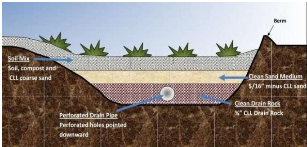
FIGURE 2.4 - TYPICAL BIORETENTION BASIN CROSS-SECTION (CLEARLAKE LAVA, N.D.)
