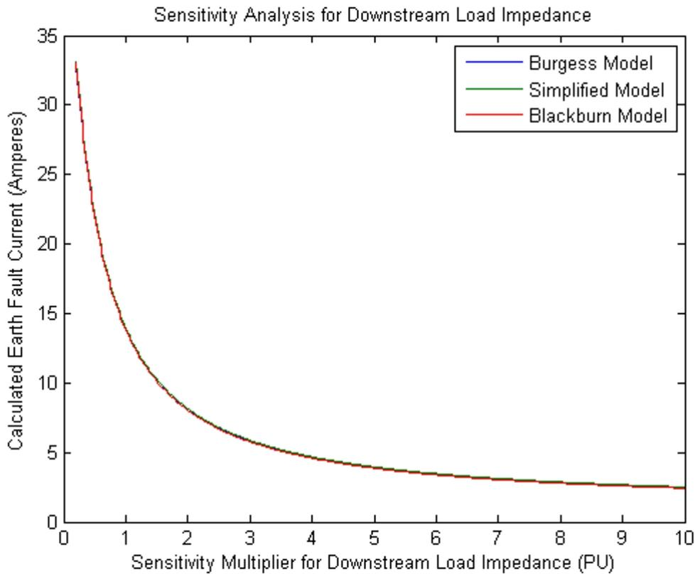
Figure 3.21: OFAT results for downstream load impedance.
