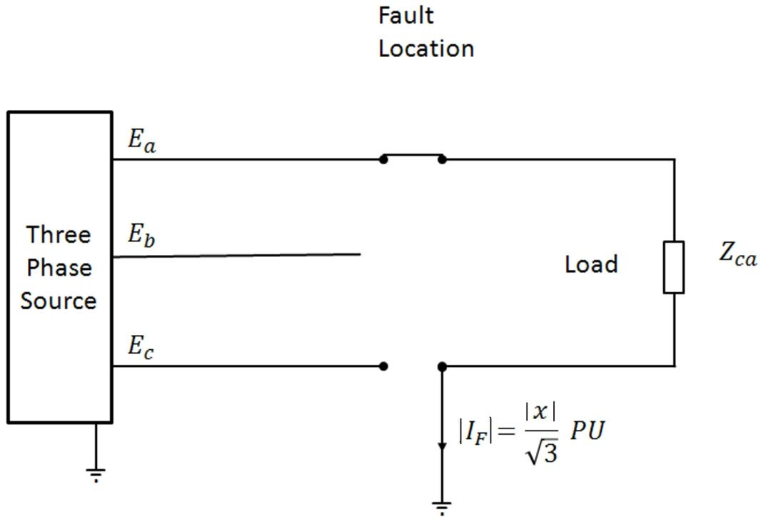
Figure 5.6: Extreme Case of Source Isolated Fault on single phase network.
