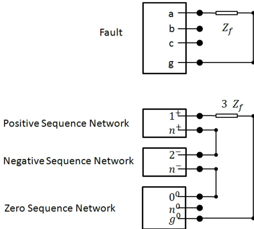
Figure 3.14: Sequence network connections diagram for phase to ground faults.
