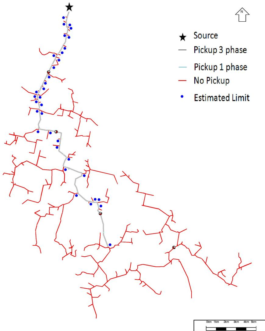
Figure 5.7: Sample 11kV rural feeder with undetectable areas shaded in red (5A SEF pickup).
