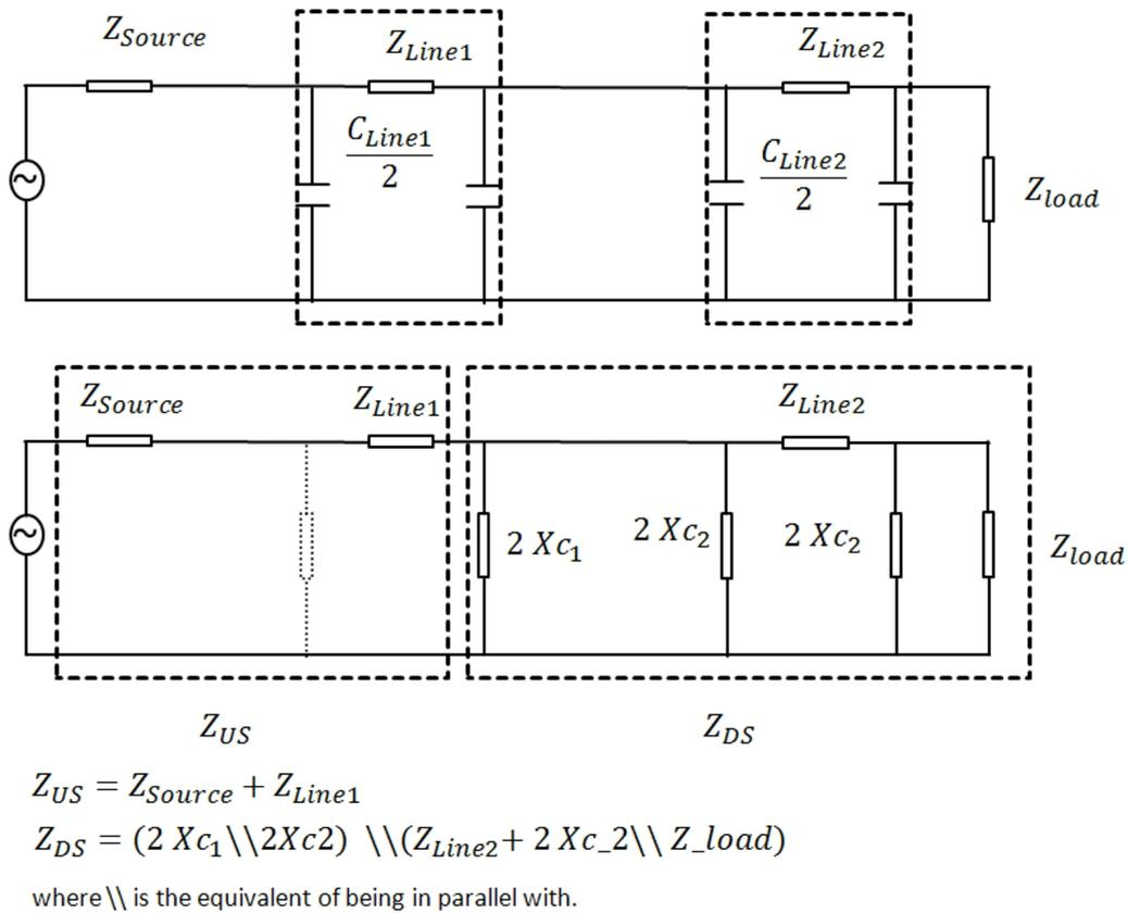
Figure 3.10: Circuit simplification to include line capacitance.
