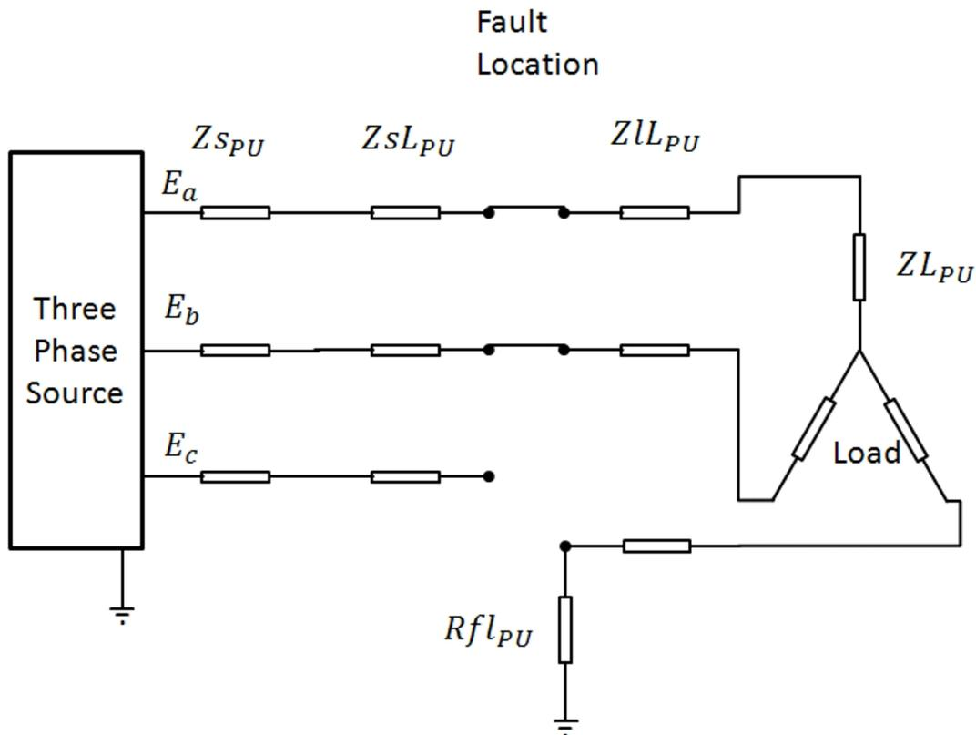
Figure 3.5: Fault schematic of Source Isolated Earth Fault with star equivalent load impedance.
