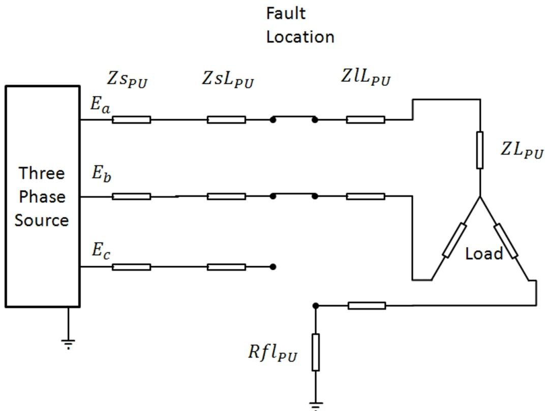
Figure 3.23: Source Isolated Earth Fault schematic.
