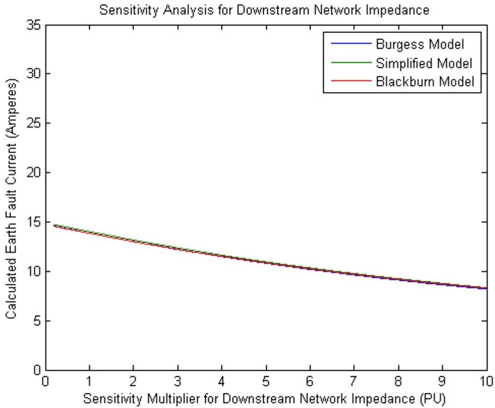
Figure 3.18: OFAT results for downstream network impedance
