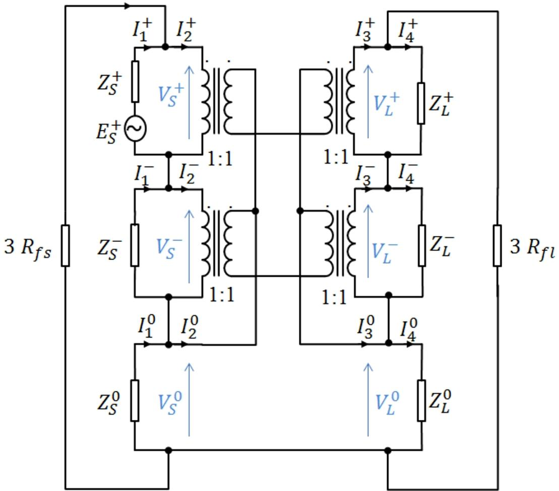
Figure 3.2: Sequence connections diagram (from the code in Burgess(2011)).
