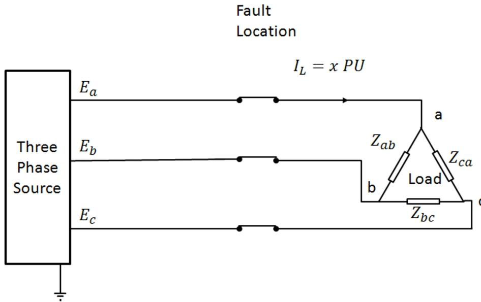
Figure 5.3: Extreme case healthy three phase network schematic.
