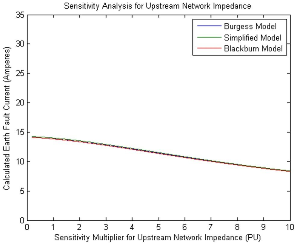
Figure 3.17: OFAT results for upstream network impedance
