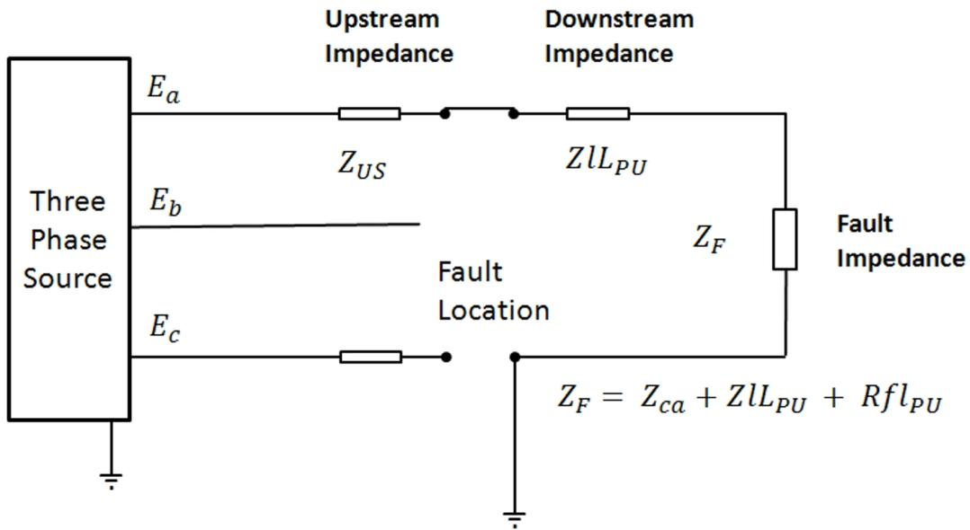
Figure 3.13: Fault schematic reduced to the equivalent of a phase to ground Fault.
