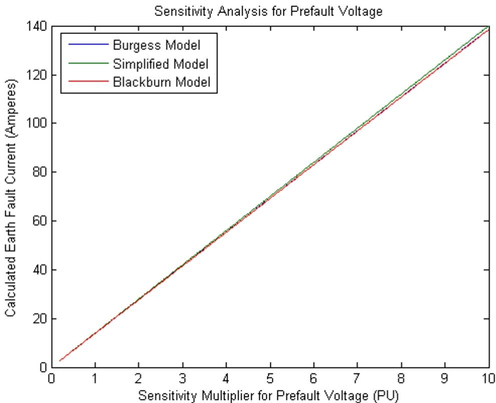
Figure 3.15: OFAT results for pre-fault voltage.
