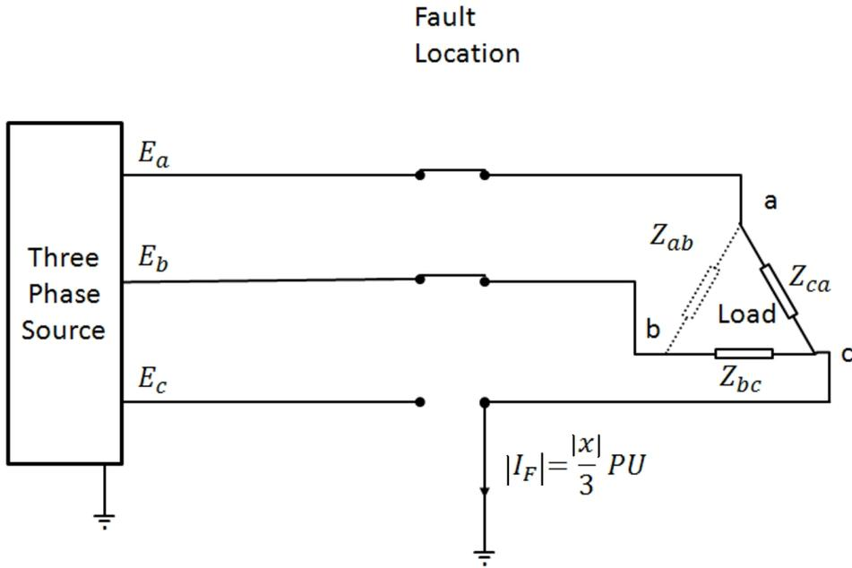
Figure 5.4: Extreme case of Source Isolated Earth Fault schematic.
