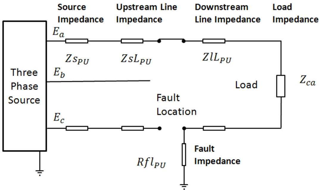
Figure 3.12: Single phase Source Isolated Earth Fault schematic.
