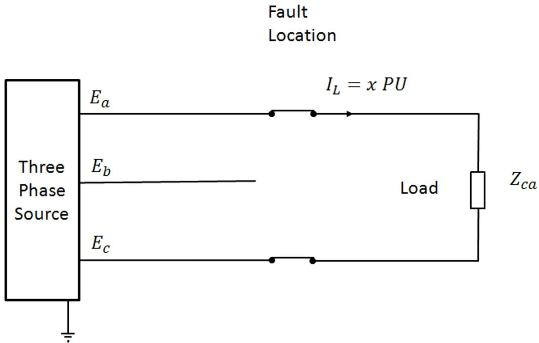
Figure 5.5: Extreme Case Single Phase Load Schematic.
