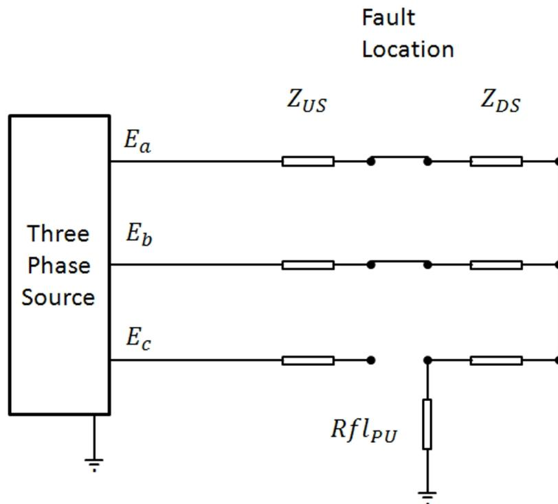
Figure 3.6: Fault schematic reduced by series addition.
