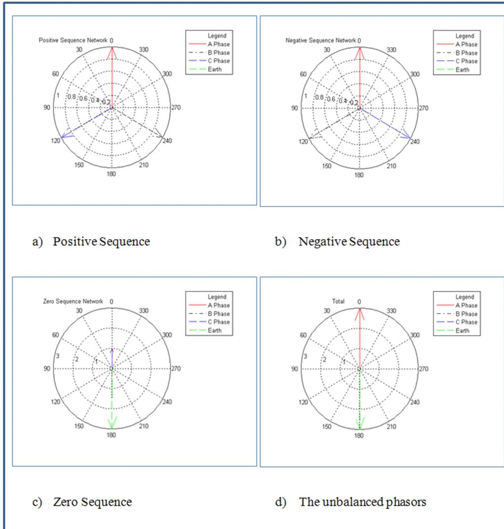
Figure 2.2: Sequence components of unbalanced phase values.
