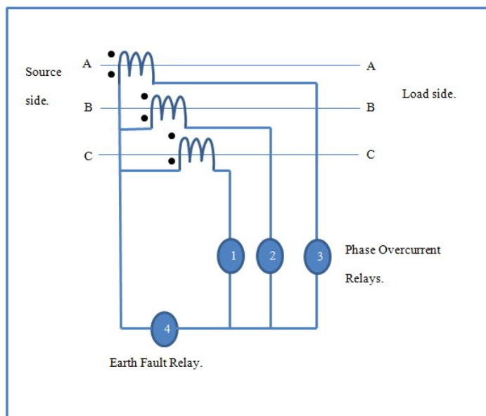
Figure 2.1: General CT arrangement for feeder CTs.
