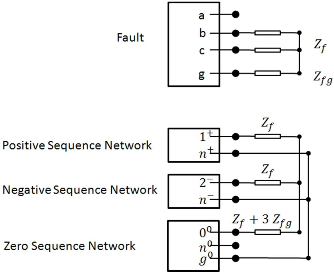
Figure 3.8: Sequence network connections diagram for phase to phase to ground faults.
