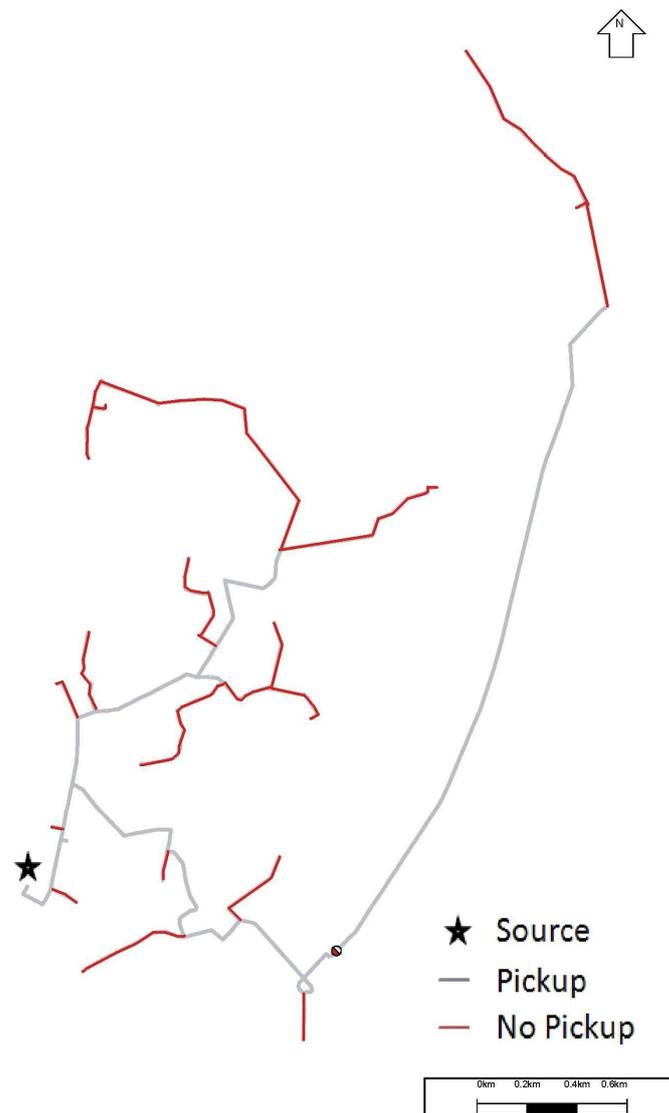
Figure 5.1: Sample CBD feeder with areas of low Source Isolated Earth Fault current highlighted in red.
