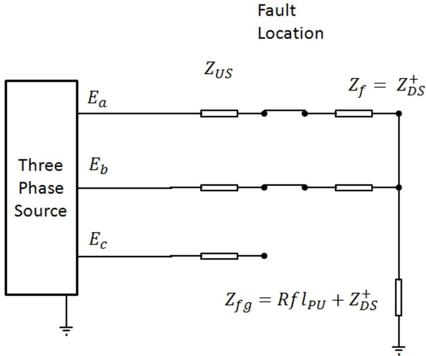
Figure 3.7: Fault schematic reduced to phase to phase to ground equivalent.
