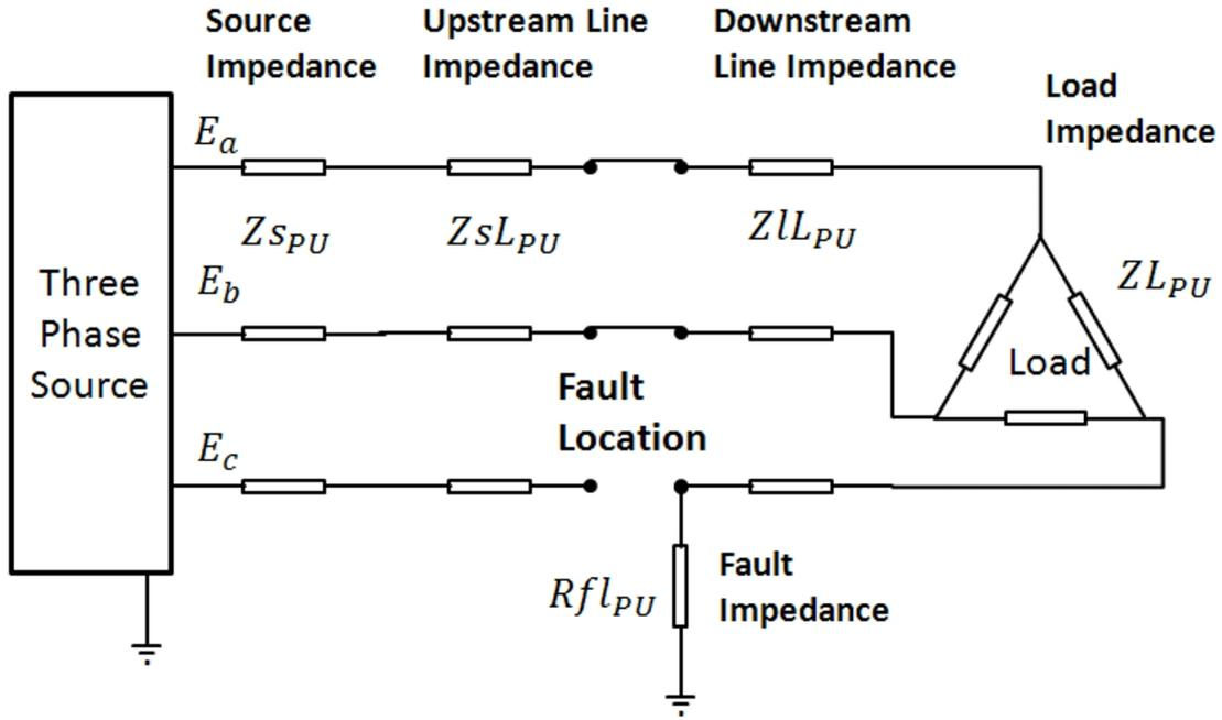
Figure 3.1: Schematic diagram of Source Isolated Earth Fault.
