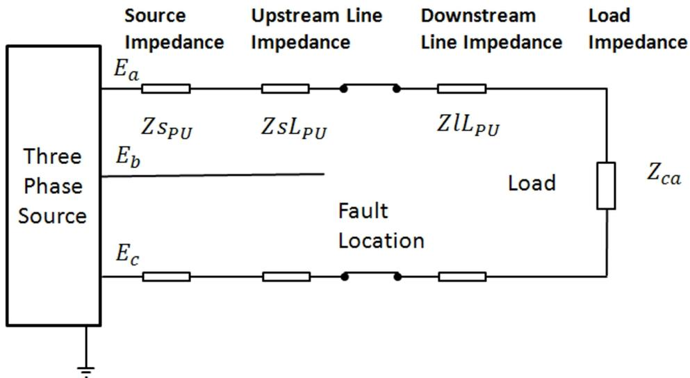
Figure 3.11: Single phase network schematic.
