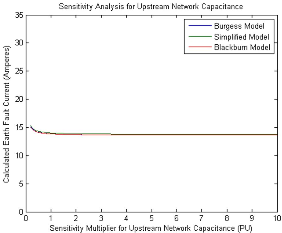
Figure 3.19: OFAT results for upstream network capacitive reactance..
