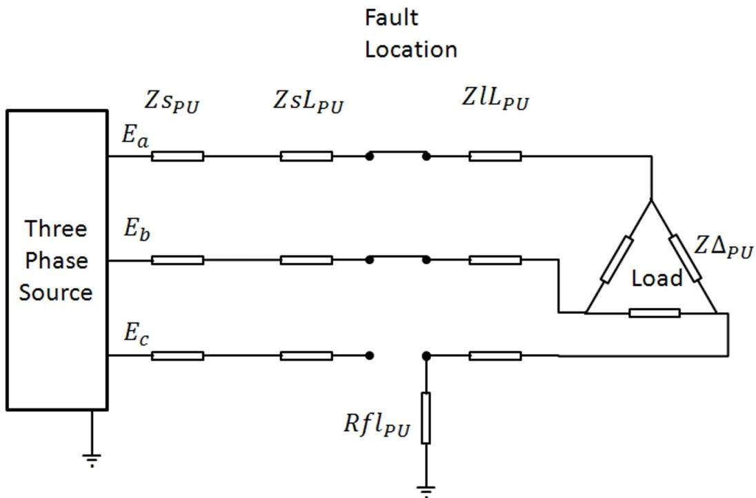
Figure 3.4: Schematic of three phase Source Isolated Earth Fault.
