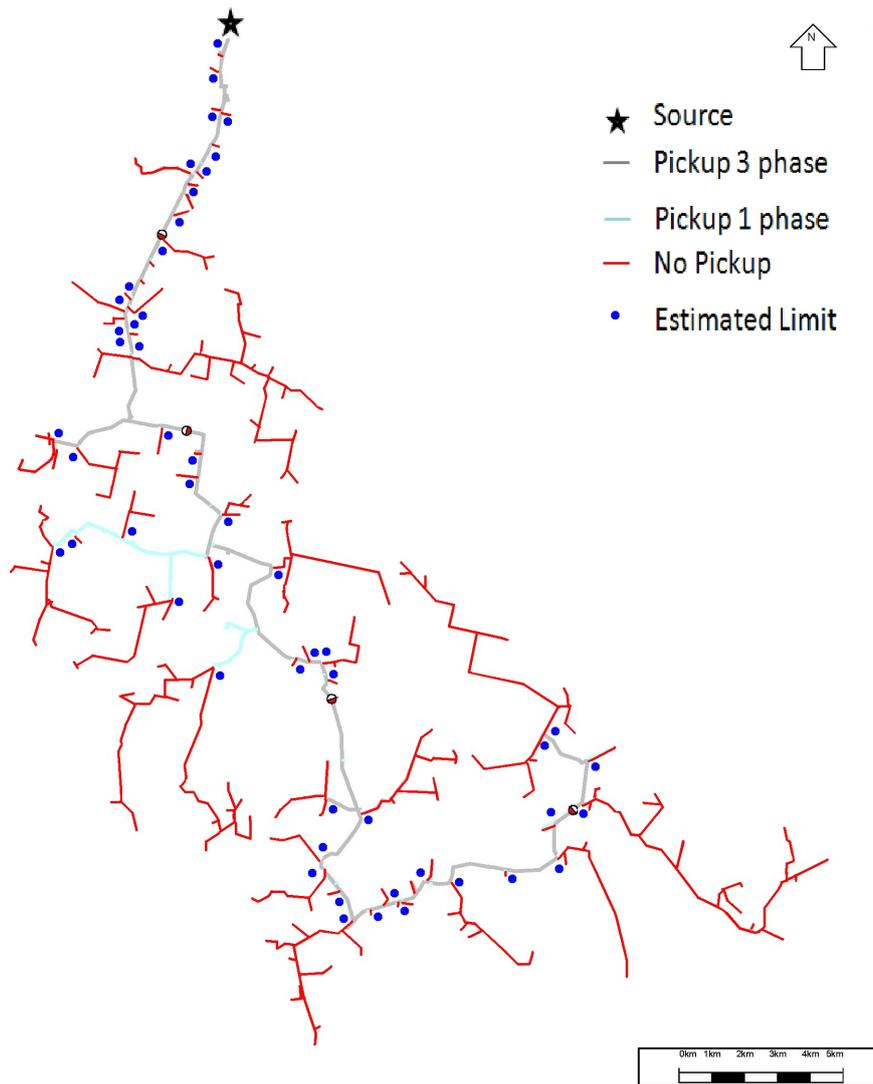
Figure 5.8: Sample 11kV rural feeder with undetectable areas shaded in red (1A SEF pickup).
