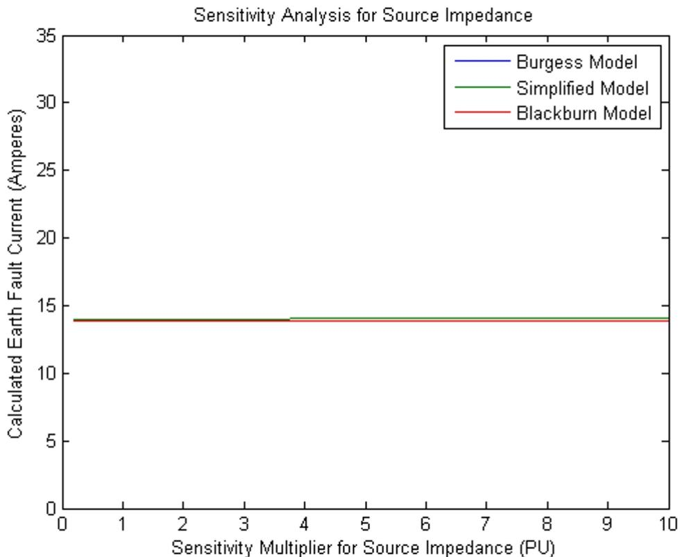
Figure 3.16: OFAT results for source impedance
