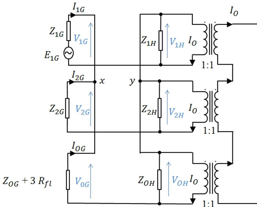
Figure 3.3: Sequence connections diagram from Blackburn(1993).
