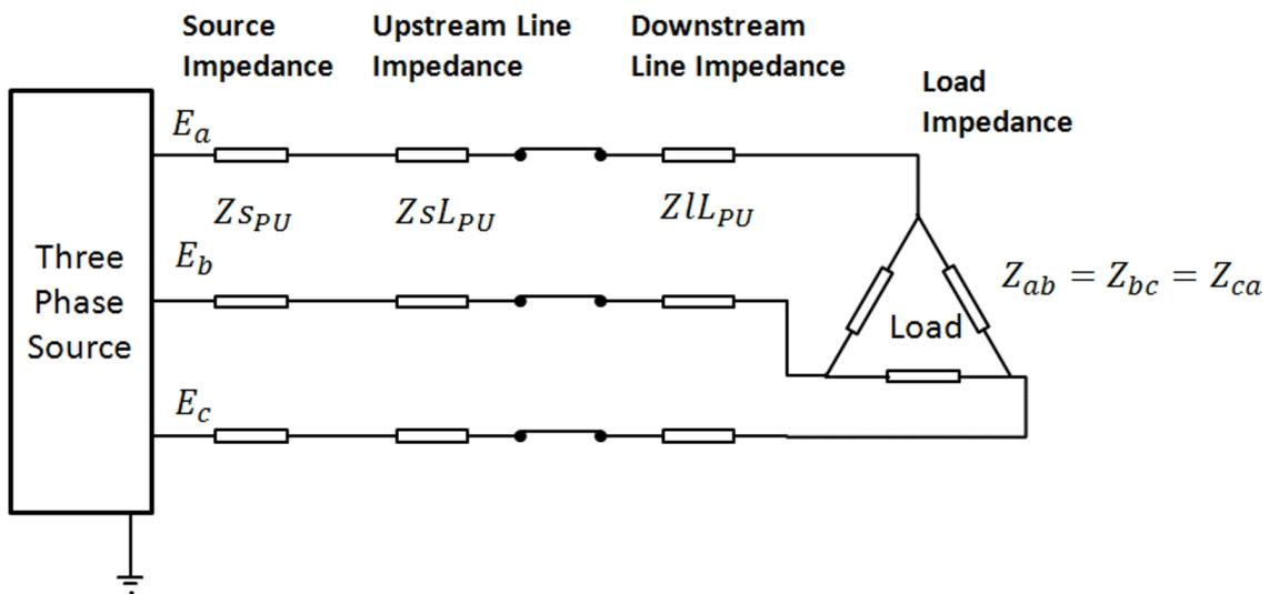
Figure 5.2: Healthy three phase network schematic.
