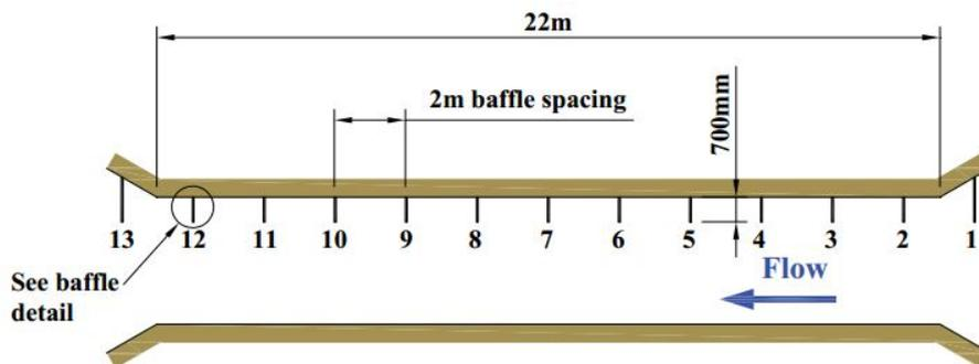
Figure 8.3: Corner 'EL' Baffle - Plan View (Kapitzke 2007)
