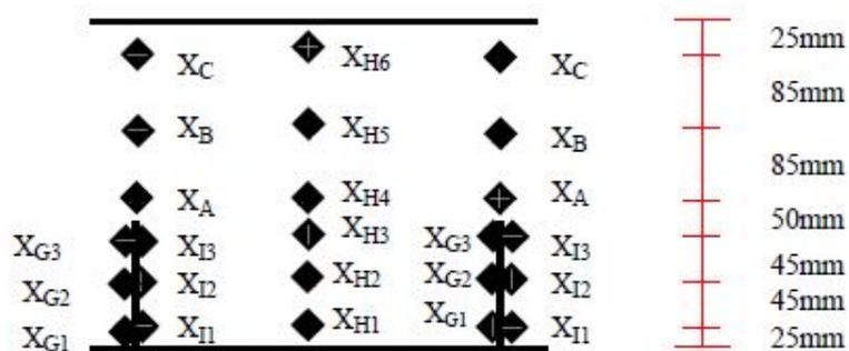
Figure 8.9: Data Collection Points for the Model Corner Baffles (Ferrando 2006)
