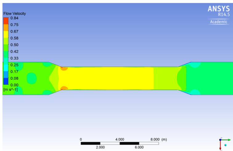
Figure 9.4: Average Flow Velocity - DAFF 'Amber' Design, 200 mm flow depth
