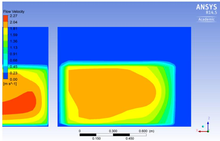
Figure 9.9: Flow Velocity - DAFF 'Red' Design mid-culvert, 500 mm flow depth
