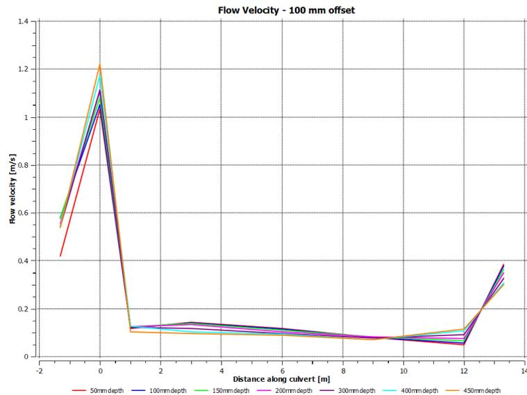
Figure 9.11: Flow Velocity Profiles - DAFF 'Red' Design, 100 mm offset from outer wall
