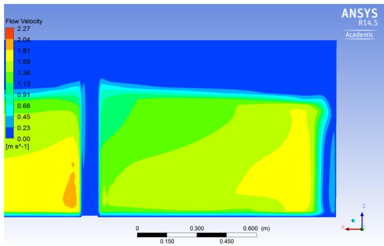
Figure 9.8: Flow Velocity - DAFF 'Red' Design culvert inlet, 500 mm flow depth
