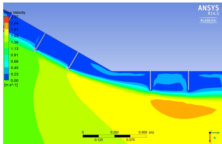
Figure 9.12: Average Flow Velocity - DAFF 'Red' Design culvert inlet, 500 mm flow depth
