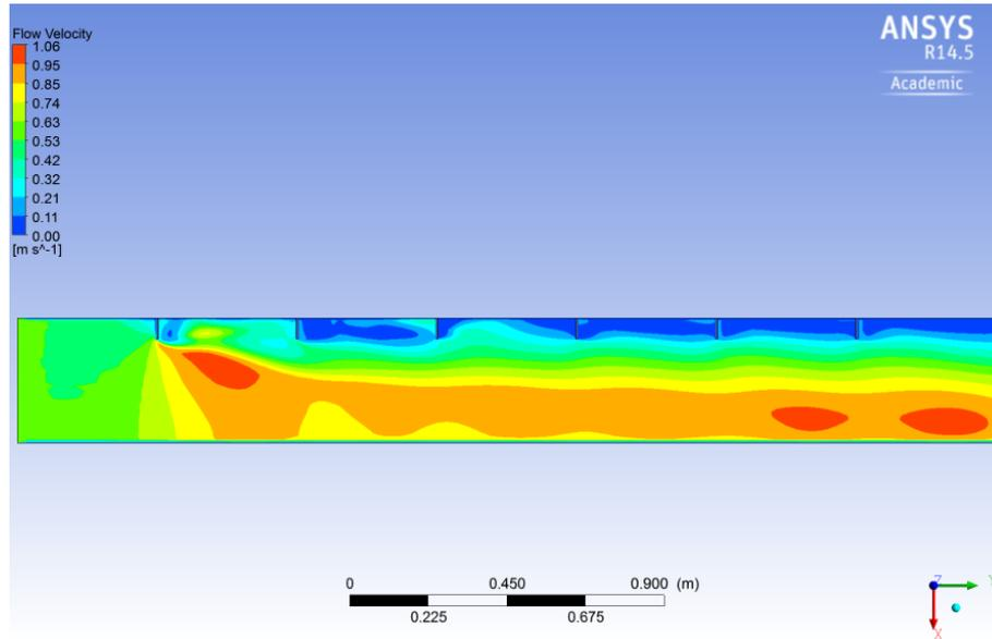
Figure 8.13: Flow velocity contour plan - laboratory model, 140 mm flow depth
