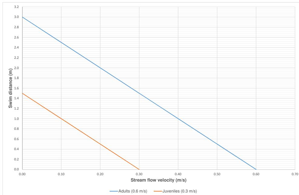
Figure 9.1: Stream flow velocity and distance travelled - Burst swim speed
