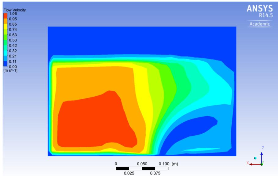
Figure 8.14: Flow velocity contour profile - laboratory model, 140 mm flow depth
