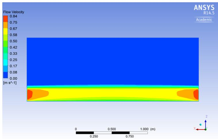
Figure 9.6: Flow Velocity - DAFF 'Red' Design culvert inlet, 200 mm flow depth
