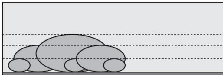
Figure 7.1: Theoretical arrangement of porous body plains for all grain sizes (Carney et al. 2006)
