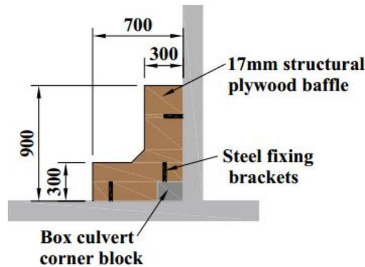
Figure 8.2: Corner 'EL' Baffle Detail (Kapitzke 2007)
