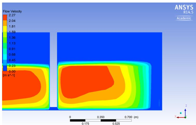
Figure 9.10: Flow Velocity - DAFF 'Red' Design culvert outlet, 500 mm flow depth
