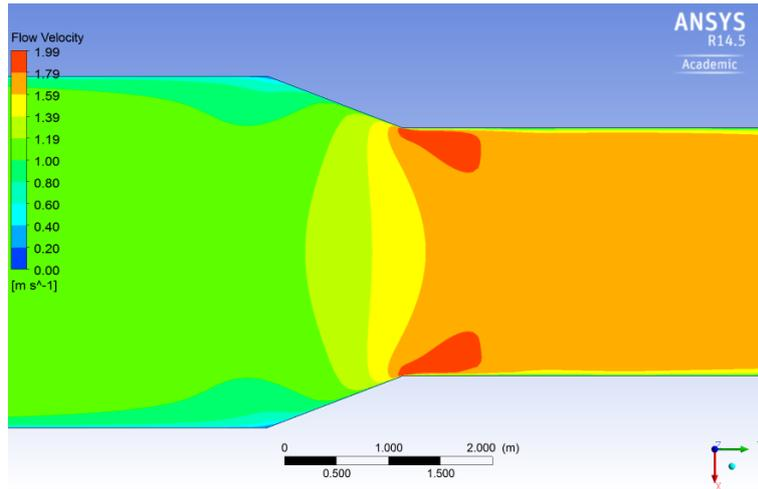
Figure 9.5: Flow Velocity - DAFF 'Red' Design culvert inlet, 500 mm flow depth
