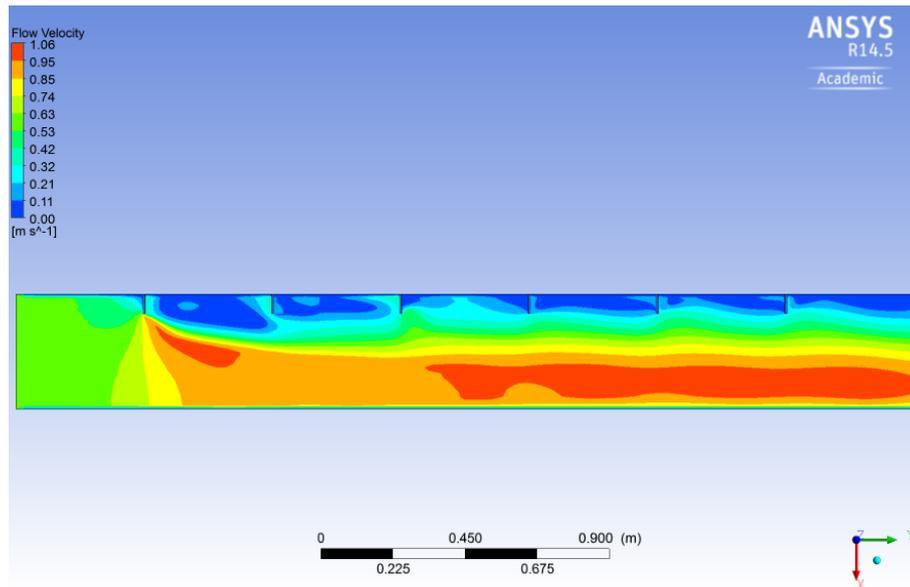
Figure 8.12: Flow velocity contour plan - laboratory model, 100 mm flow depth
