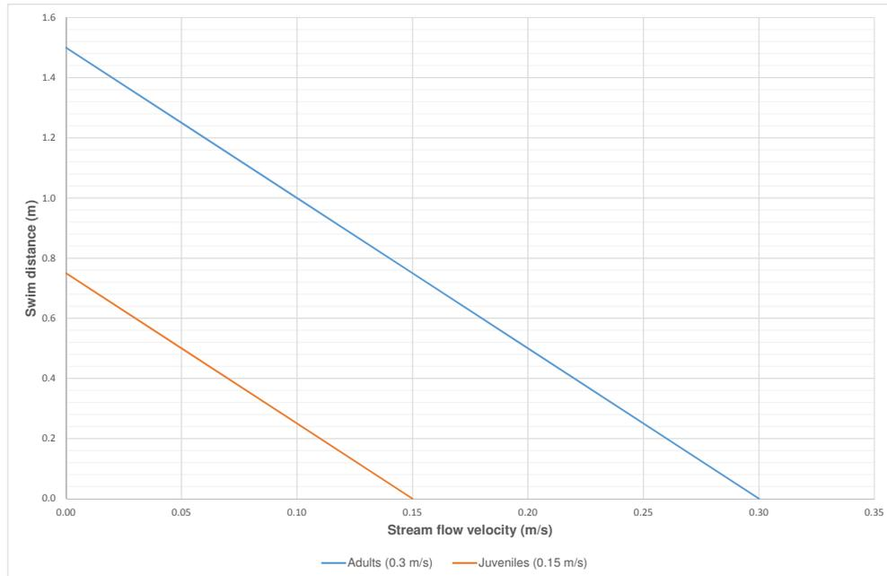
Figure 9.2: Stream flow velocity and distance travelled - Prolonged swim speed
