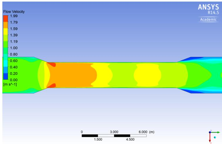
Figure 9.3: Average Flow Velocity - DAFF 'Amber' Design, 500 mm flow depth
