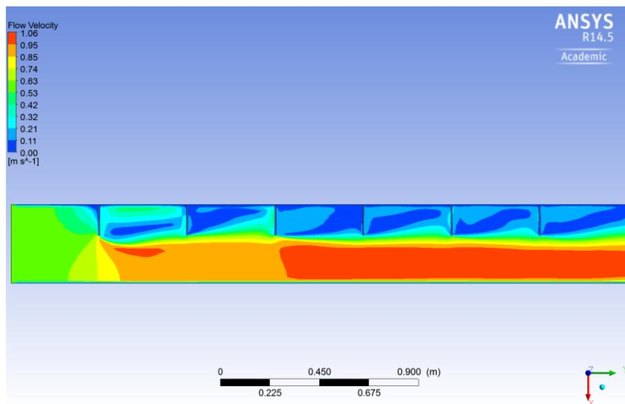
Figure 8.10: Flow velocity contour plot - laboratory model, 30 mm flow depth
