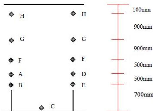
Figure 8.5: Data Collection Points for the Prototype Corner Baffles (Ferrando 2006)
