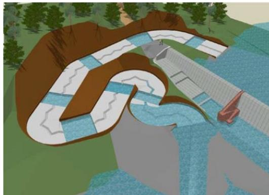
Figure 5.1: Proposed natural bypass fish passage layout (Delaere et al. 2011)
