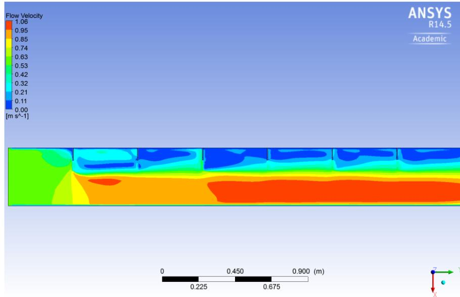
Figure 8.11: Flow velocity contour plan - laboratory model, 60 mm flow depth
