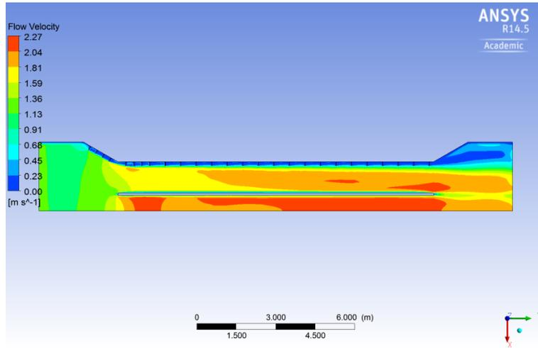
Figure 9.7: Average Flow Velocity - DAFF 'Red' Design, 500 mm flow depth
