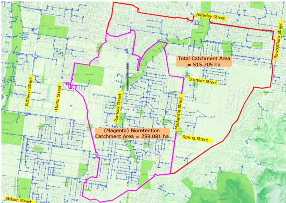
Figure 4.21 – Bioretention catchment area shown within WBH catchment
