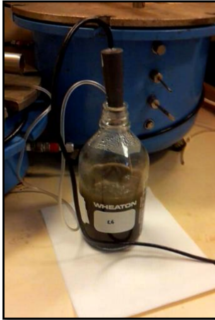
Figure 8 Test Bottle being Sparged while Measuring Oxygen Levels
