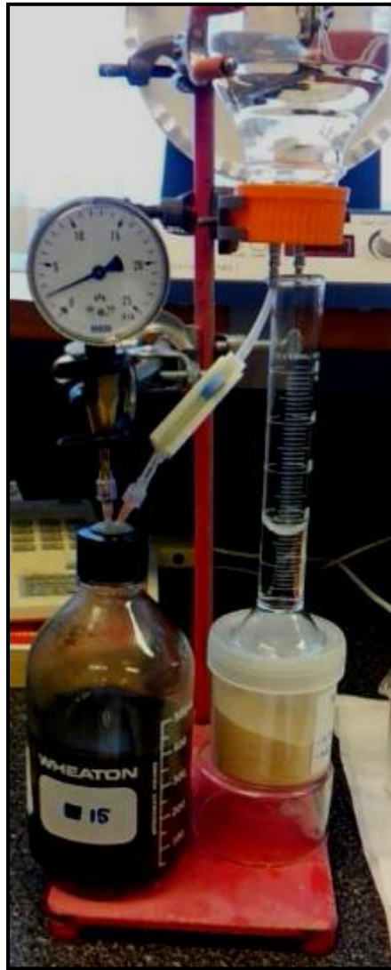
Figure 10 Biological Methane Potential Assay Apparatus
