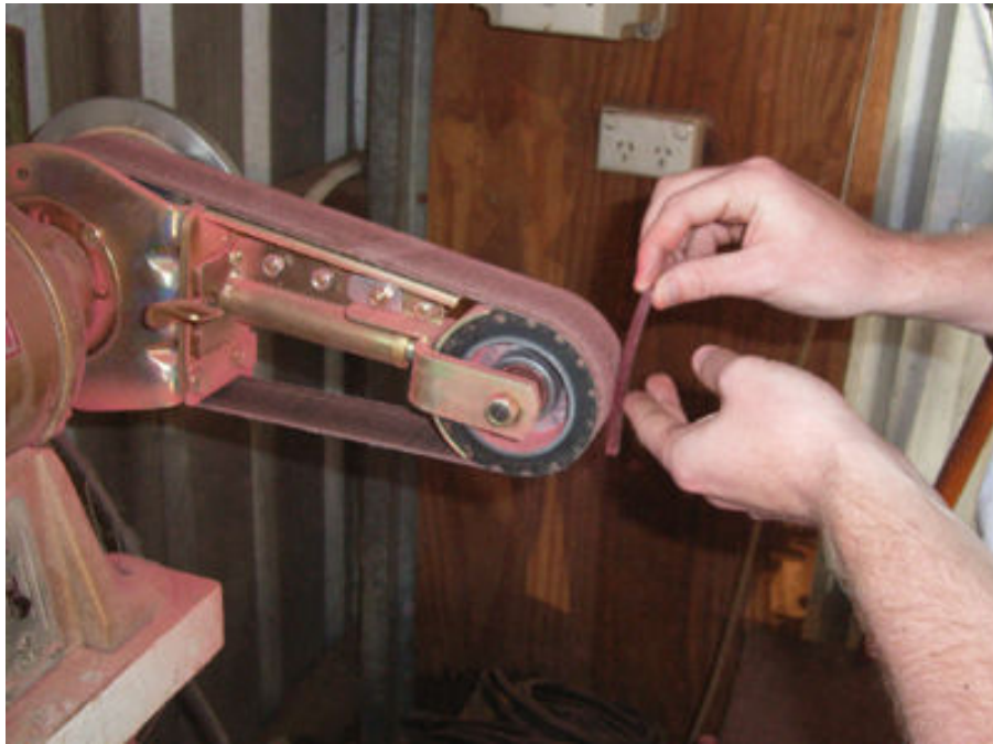
Figure 14: Removal of porosity
