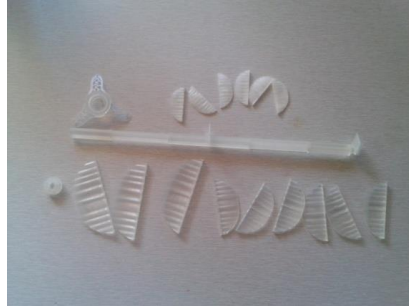
Figure 3.1.2c Finished clean turbine parts
