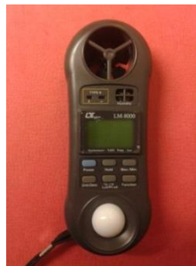
Figure 2.4a Weather multi-meter including anemometer
