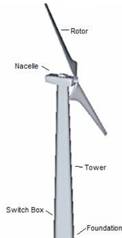
Figure 2.3.1a 3D model of a wind turbine through using the program Google Sketch up 8.
