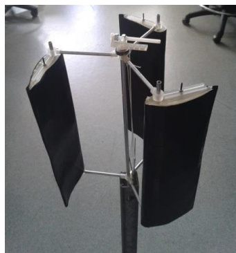
Figure 4.3.3h– Finish wind turbine – ready for testing
