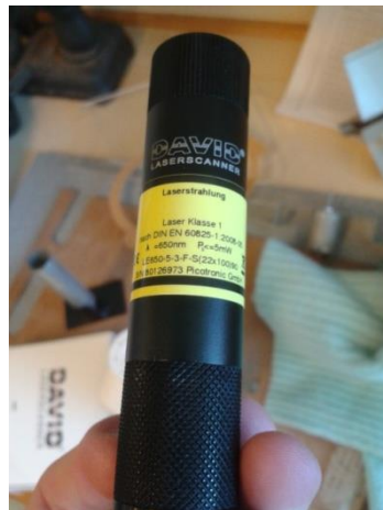
Figure 3.2.1k – David's 3D laser scanner laser module
