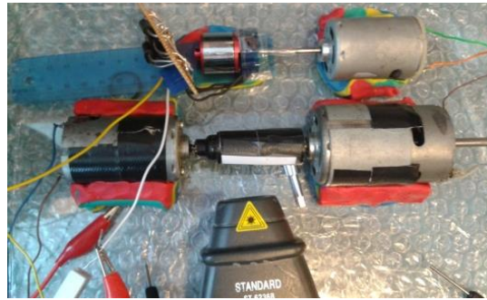
Figure 3.1.3.h – TOP: three-phase generator, MID: PMDC machine, BOTTOM: tachometer
