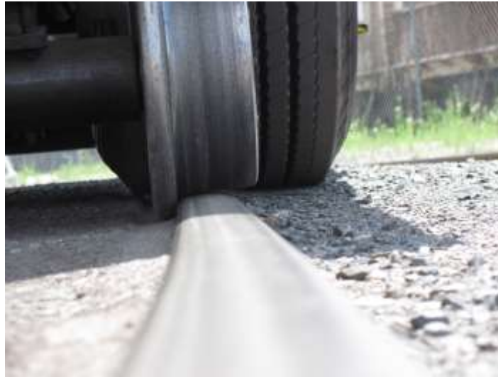
Figure 4-3: Tyre supported by roadway
