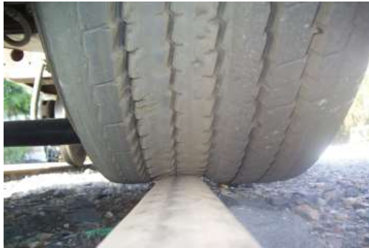
Figure 4-12: DN 300 tyre wear
