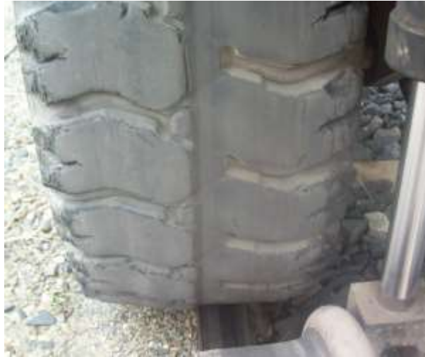
Figure 4-13: DN 100 tyre wear
