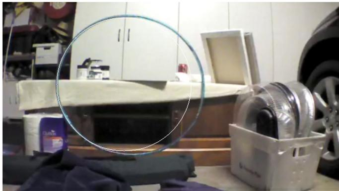
Figure 4.3: Finding a Hoop with *cvHoughCircle*
