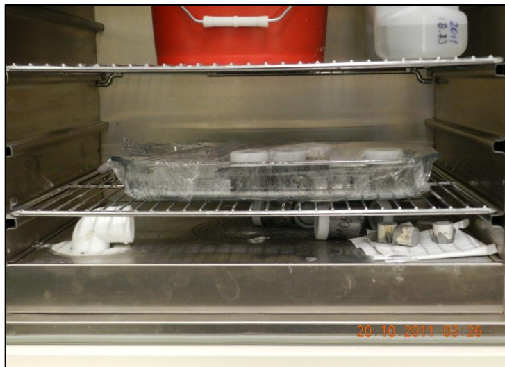
Figure 24: Container covered with plastic for curing
