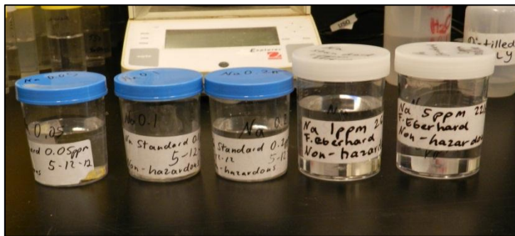
Figure 40: Sodium (Na) standard solutions
