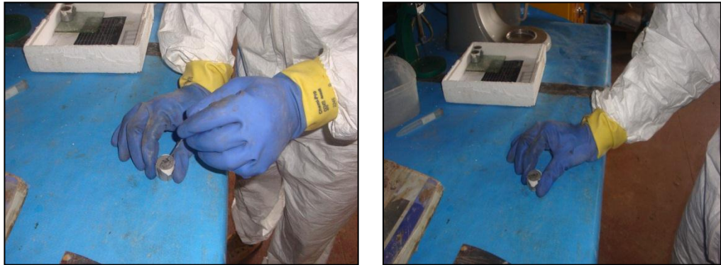
Figure 23: Compacting of geopolymer paste
