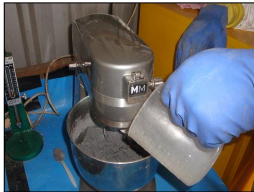
Figure 19: Alkali Activator being added to fly ash
