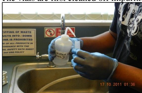
Figure 38: Vial cleaned with distilled water
