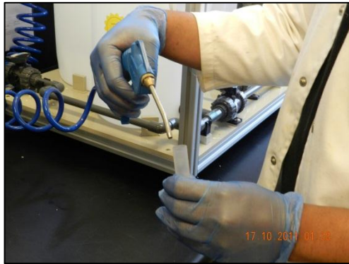
Figure 39: Vial being dried with compressed air
