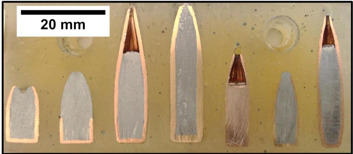
Figure 6.1-3 Projectile cross section from left .30 cal (90 gr XTP, 100 gr SP, 155 gr Berger, 200 gr Woodleigh) .22 cal (50 gr Barnes, 55 gr Speer, 90gr Berger)
