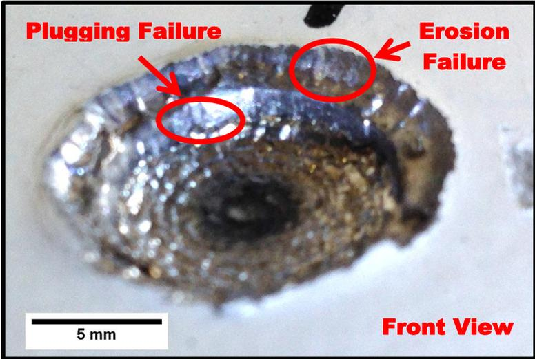
Figure 6.3-1 Crater failure zones front view
