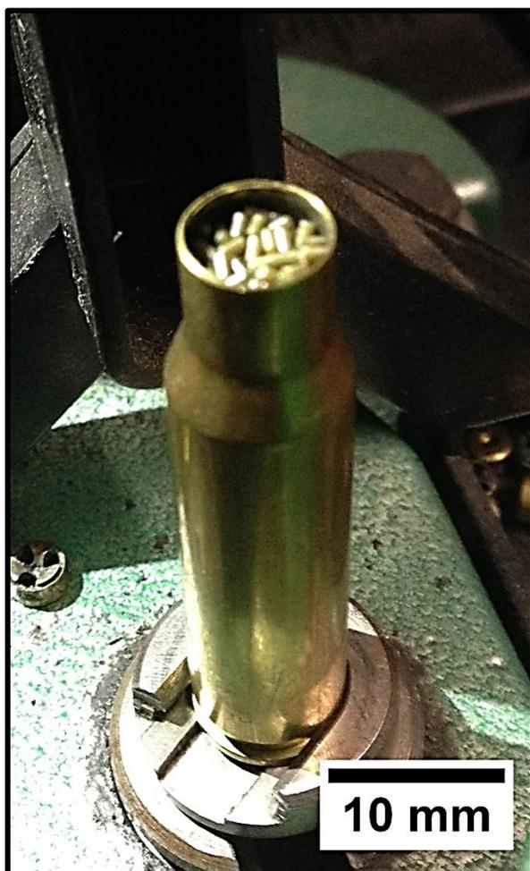
**Figure 4.2-1 .30 cal 90 gr at Max case capacity**
