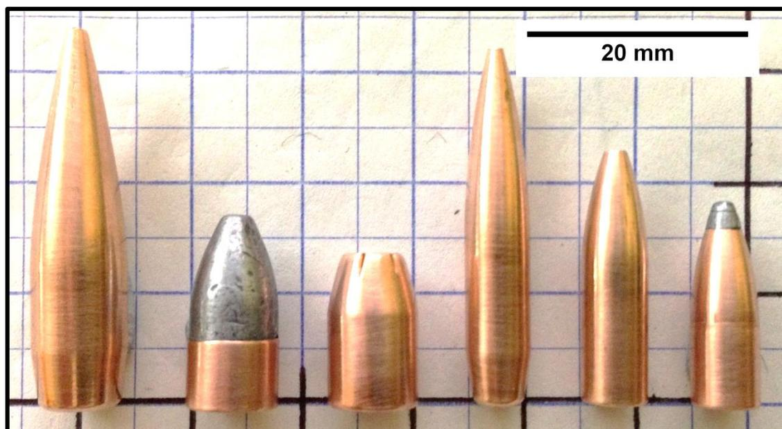
**Figure 4.1-3 Projectiles, from left .30 cal (155gr, 100gr, 90gr) & .22 cal (90gr, 50gr, 55gr)**
