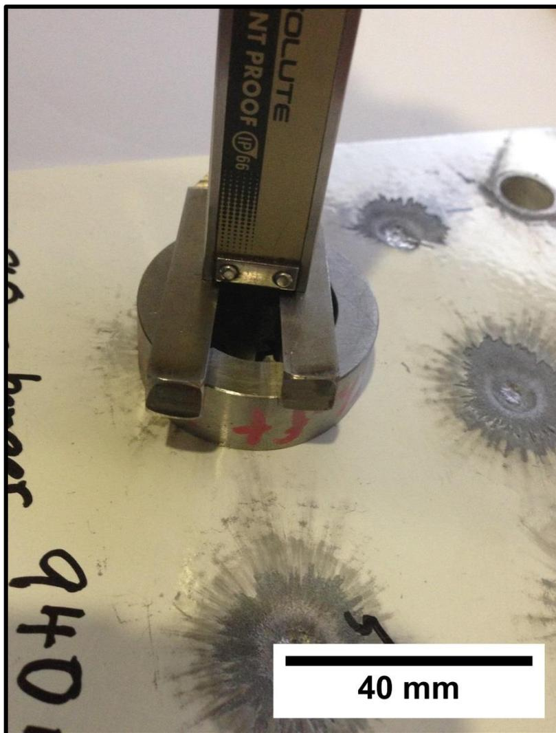
Figure 4.3-1 Measuring penetration depth
