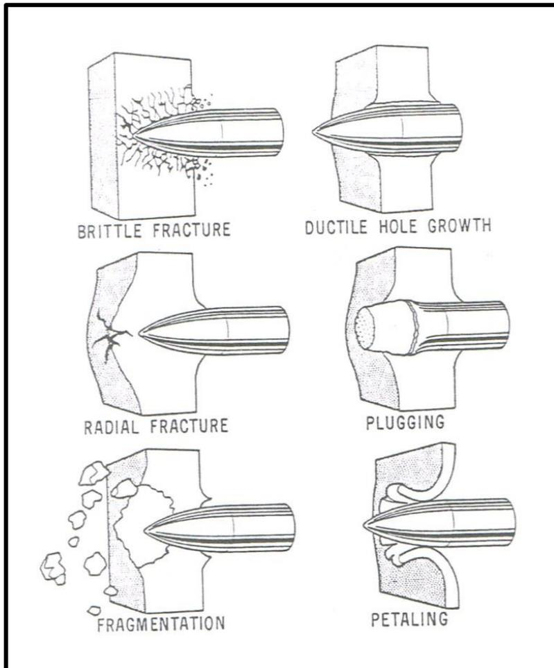
**Figure 2.6-1 Failure modes Roesneberg, Dekel (2012)**
