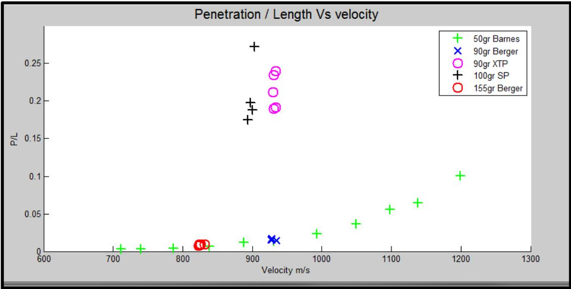
Figure 6.1-2 P/L Vs velocity
