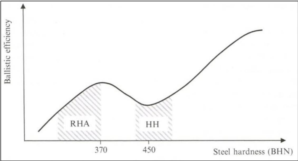
Figure 2.7-1 Ballistic efficiency vs. hardness (Dekel & Rosenberg, 2012)
