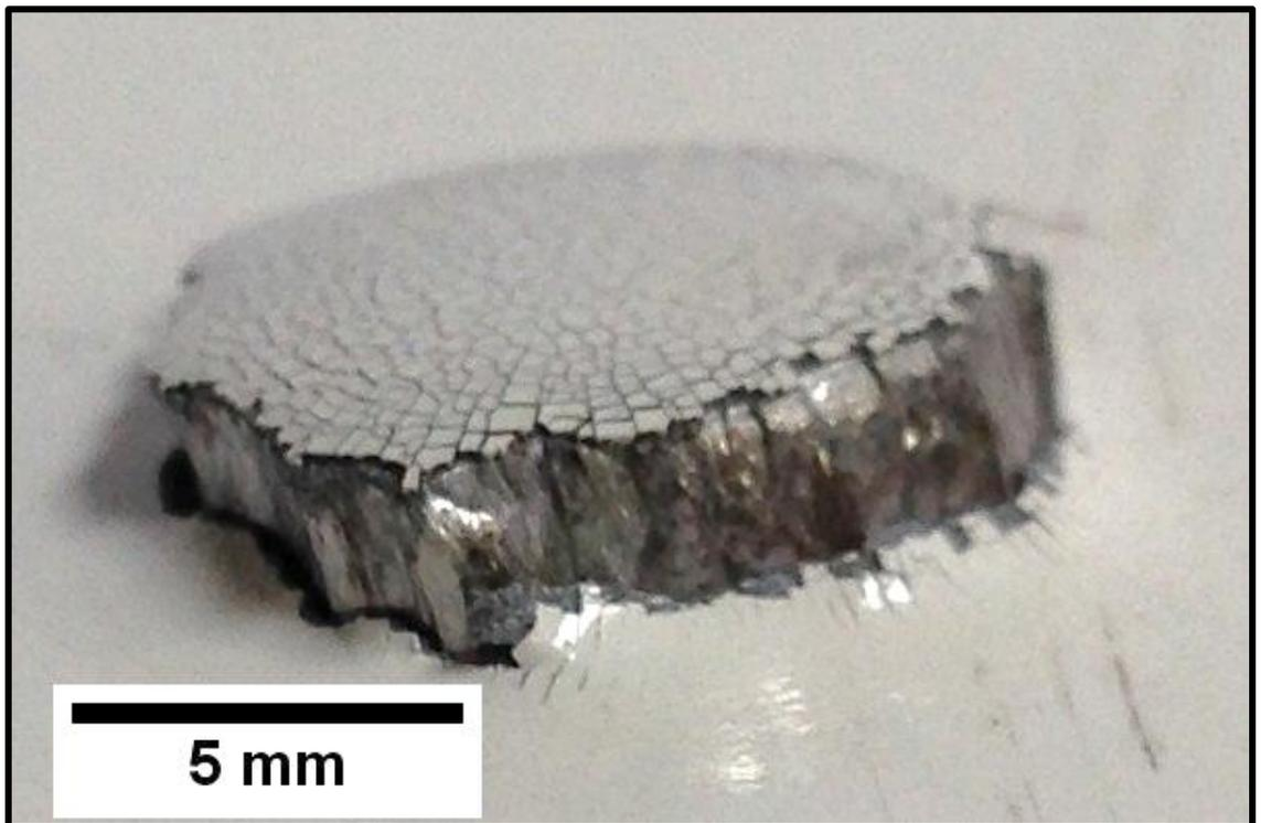
Figure 5.4-3 30 cal 100gr Hornady rear of plate
