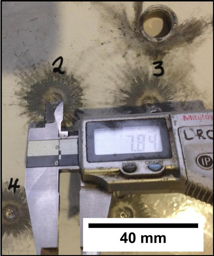
Figure 4.3-2 Measuring penetration and crater diameter
