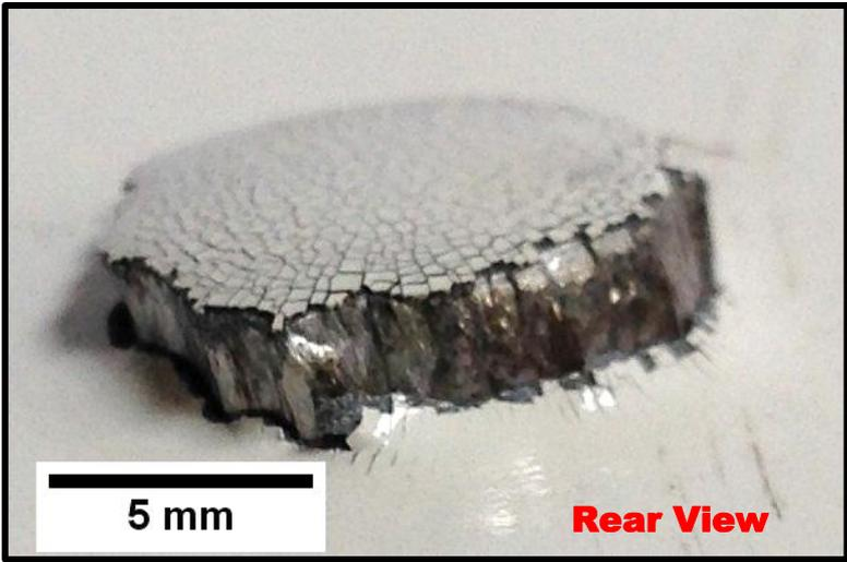
Figure 6.3-2 Crater failure zones rear view
