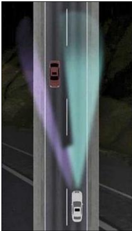
Figure 2.18: Toyota High Beam Filter Technology Source: (Automotive News 2013)
