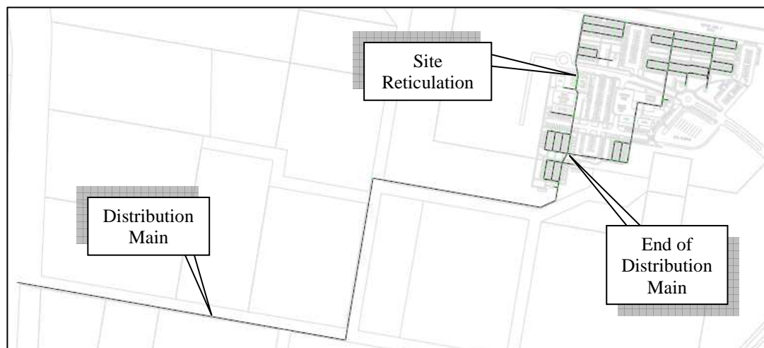
Figure 3.2a Water Supply Network Layout – Entire Layout
