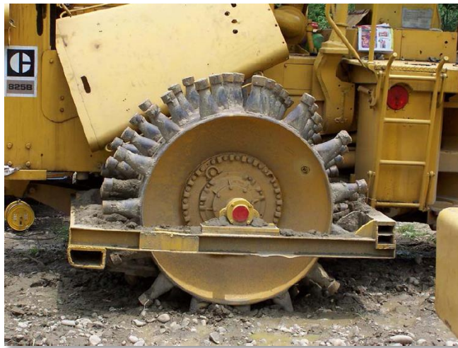
Figure 2.16: Type of sheepsfoot roller used for compacting clayey soils (USBR 1984)
