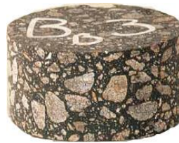
Figure 2.12: Core sample of Asphalt Concrete (AC) dam core
