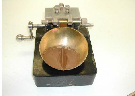
**Figure 12 - Apparatus for Casagrande liquid limit test (Earl 2010)**
