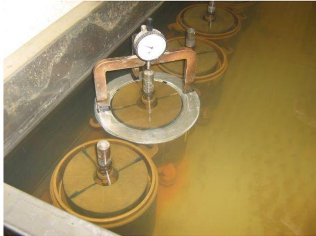
**Figure 9 - CBR test specimens with swell measurement apparatus (Walters 2008)**
