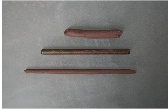
**Figure 14 - Plastic limit test specimens adjacent to 3mm diameter guide rod (Earl 2010)**
