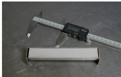
**Figure 15 - Soil specimen in linear shrinkage test mould (Main Roads 2008)**
