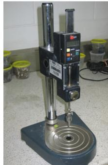
**Figure 13 - Apparatus for fall cone liquid limit test (TMR 2013)**
