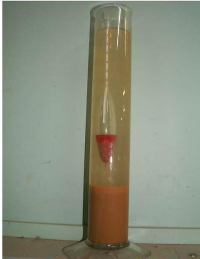
**Figure 10 - Hydrometer Testing (Earl 2005)**
