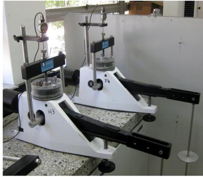
**Figure 17 - Apparatus (Oedometer) for swell tests**
