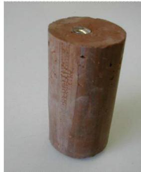
Figure 16 - Core shrinkage specimen
