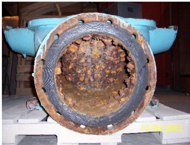
Figure 5: Pump internal with severe tuberculation (Verosky et al. 2008).
