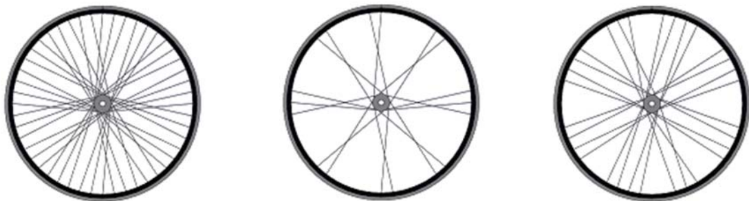
Figure 4.2-6. 48 spoke wheel optimised spoke geometry - (left) full wheel; (centre) 18 LH spokes; (right) 30 RH spokes.
