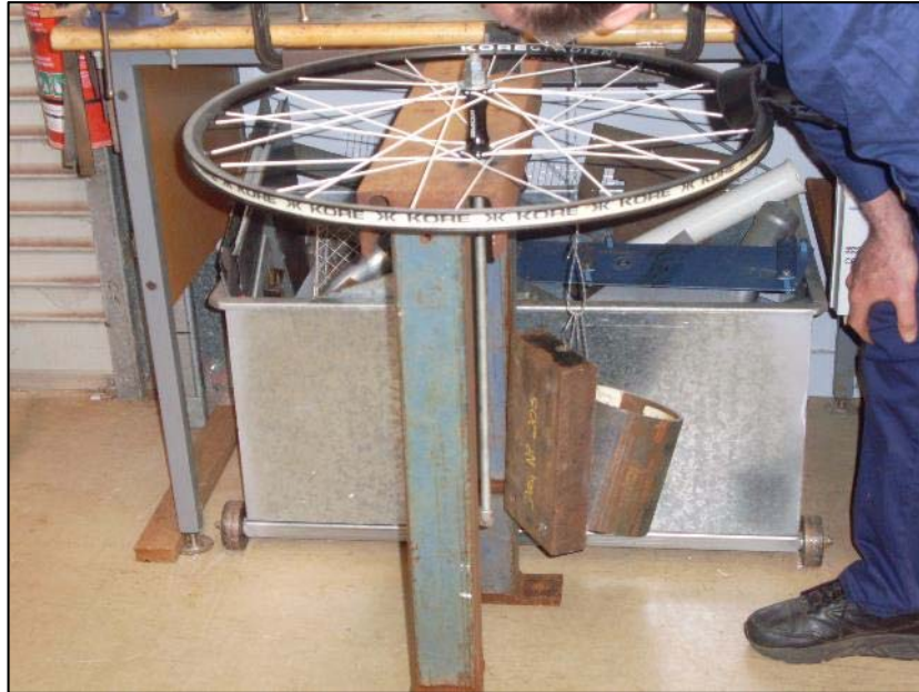
Figure 3.5-2. The application and deformation measurement of the 92.4 N lateral load. Photo courtesy of Peta Keller (2013).
