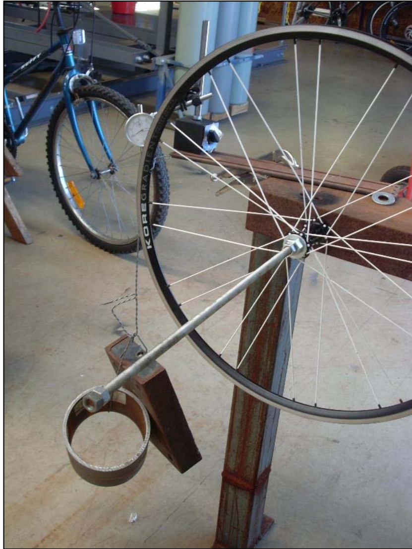
Figure 3.5-3. The application and deformation measurement of the 92.4 N tangential load. Photo courtesy of Peta Keller (2013).
