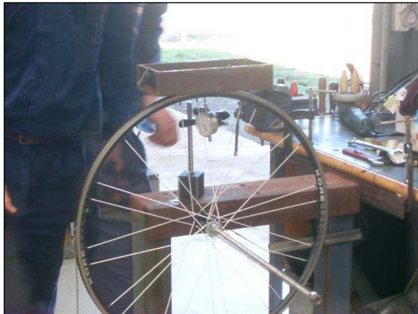
Figure 3.5-1. The application and deformation of the 44.9 N radial load.
