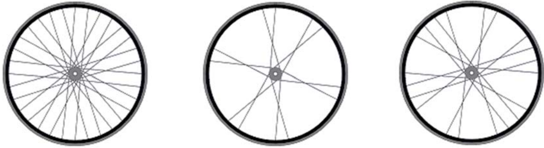
Figure 4.2-4. 32 spoke wheel optimised spoke geometry - (left) full wheel; (centre) 12 LH spokes; (right) 20 RH spokes.
