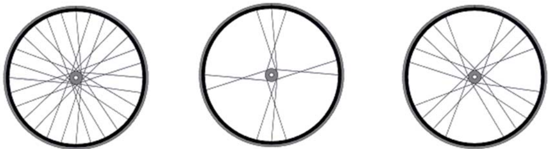
Figure 4.2-3. 28 spoke wheel optimised spoke geometry - ( left ) full wheel; ( centre ) 10 LH spokes; ( right ) 18 RH spokes.
