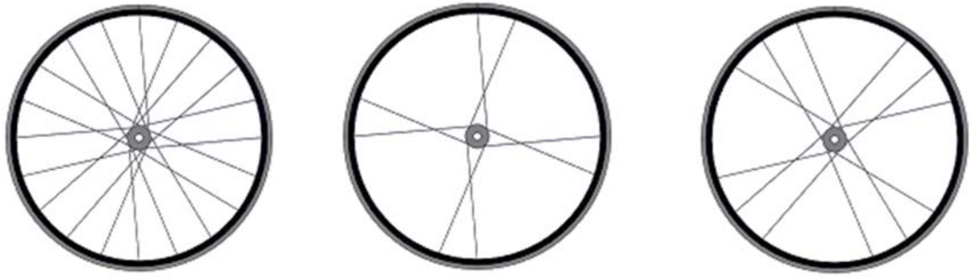
Figure 4.2-1. 20 spoke wheel optimised spoke geometry - ( left ) full wheel; ( centre ) 8 LHS spokes; ( right ) 12 RH spokes.
