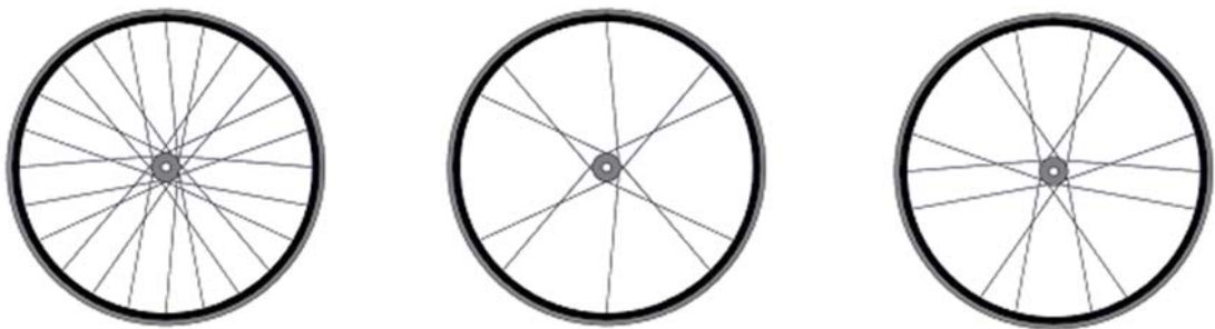
Figure 4.2-2. 24 spoke wheel optimised spoke geometry - ( left ) full wheel; ( centre ) 10 LH spokes; ( right ) 14 RH spokes.
