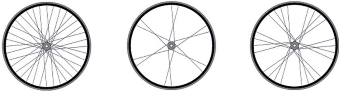
Figure 4.2-5. 36 spoke wheel optimised spoke geometry - (left) full wheel; (centre) 12 LH spokes; (right) 24 RH spokes.
