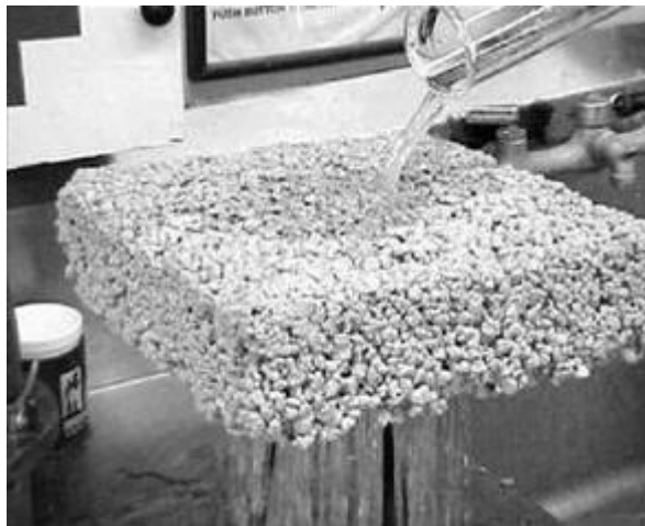
Figure 3.3 - Demonstration of water passing through porous concrete (National Ready Mix Concrete Association 2004)
