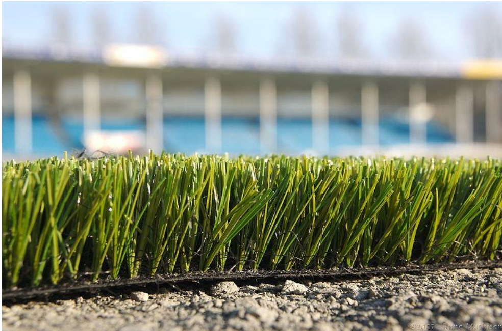
Figure 5.1: Cross section of typical artificial turf used in sporting pitches (Mathisen 2007)
