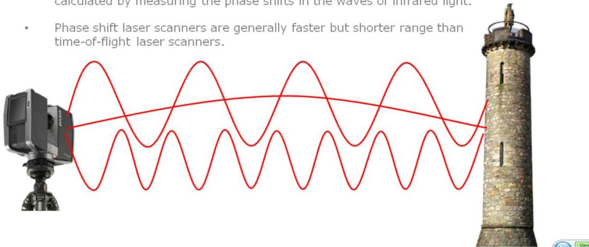
**Figure 2** An example of a Phase based laser scanner. Source Geomatics.
