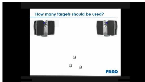
**Figure 9** three targets required for registration as a minimum (FARO).
