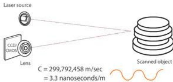
**Figure 3** How the laser scanner works.
