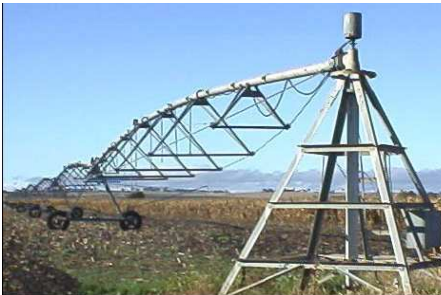
Figure 4: Centre Pivot Irrigation System Source: Foley 2001.
