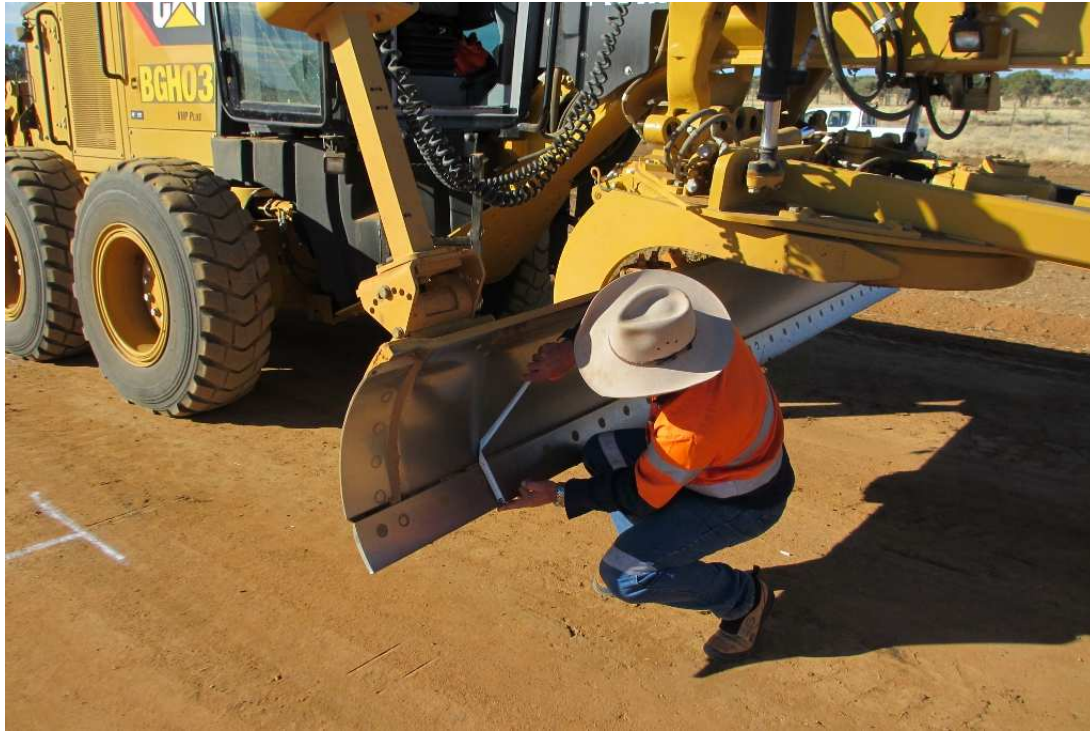
Figure 8-3 Measuring Blade Wear Landsborough Highway
