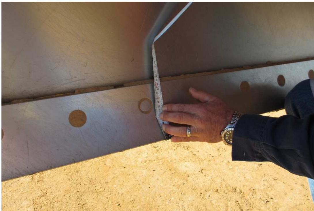
Figure 8-4 Measuring Blade Wear Landsborough Highway
