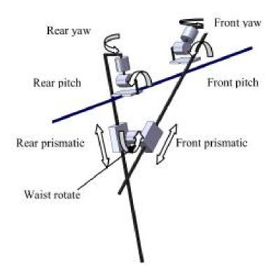
Figure 2.3: Structure of a line walking robot (L.Wang, 2010)
