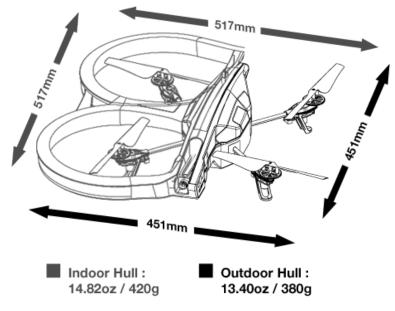
Figure 4.1: AR Drone Specifications
