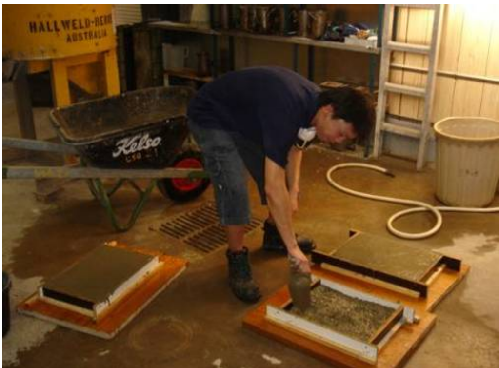
Figure 2.28: Pure concrete into the mold.
