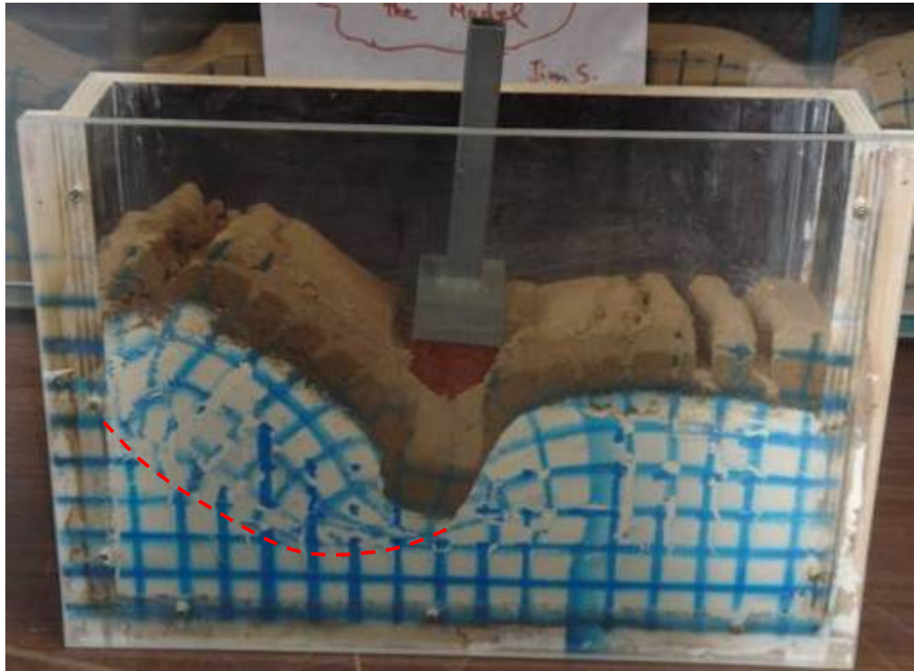
Figure 2.25: Failure mechanism of sand on clay model.
