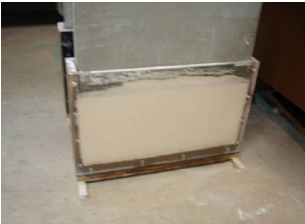
Figure 2.34: Settlement after applied the second concrete block.
