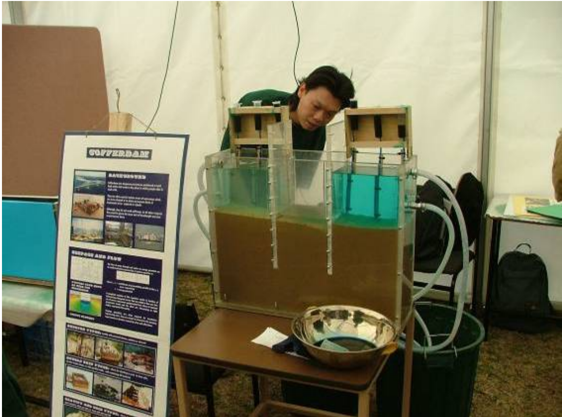
Figure 4.12: Setting the cofferdam model.
