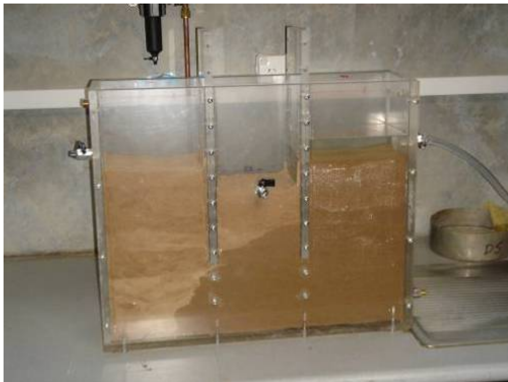
Figure 3.14: Fill up the water and saturated the sand sample.
