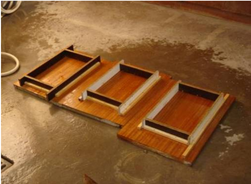
Figure 2.27: Mold for casting the concrete block.
