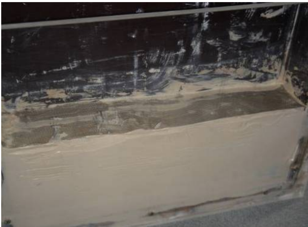
Figure 2.17: Soil reinforcement of sand on clay model.
