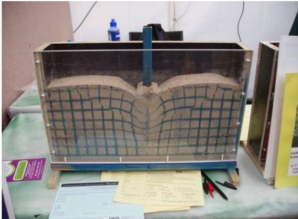
Figure 4.11: Revealed failure patterns.
