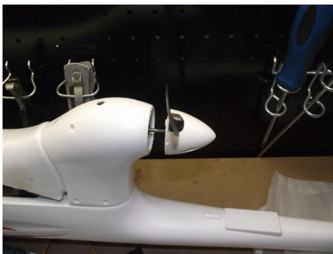
Figure 8.1 – Aircraft propeller capable of speeds of up to 10000 RPM.
