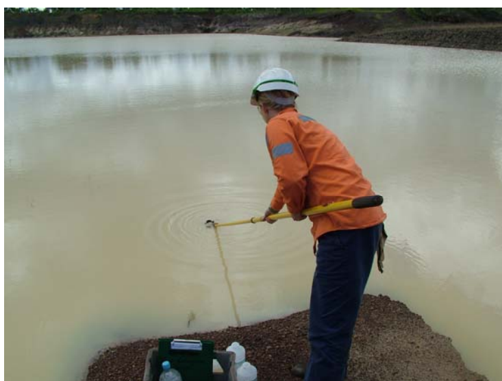
Figure 3.1: Collection of Sample Water
