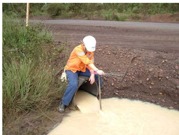
Flocculant block is held in place with survey peg. Instant clarification is not evident.
