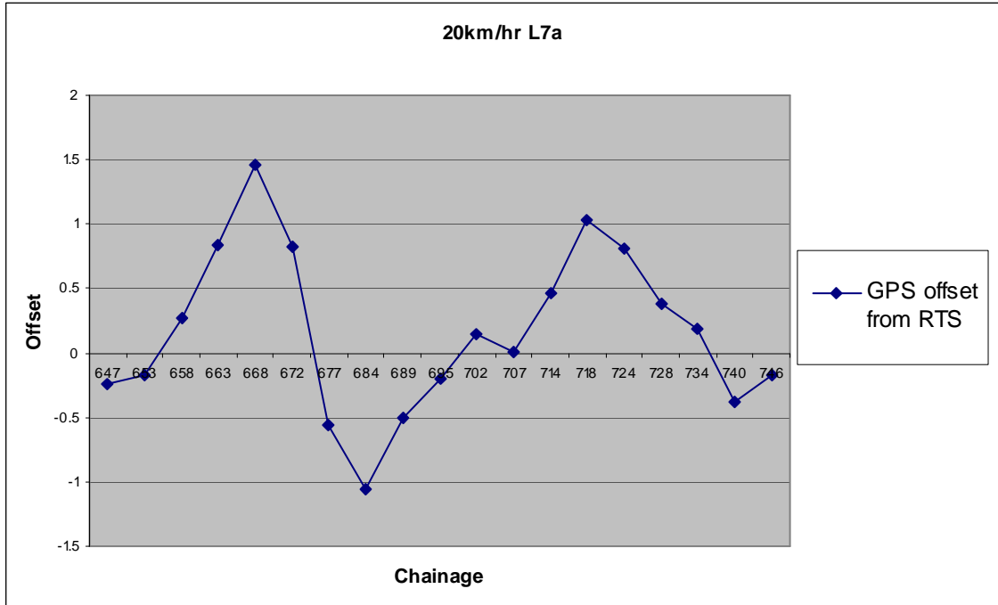
Figure D.7: Comparison between RTS and GPS Dynamic Tracking measurements at 20km/hr.
