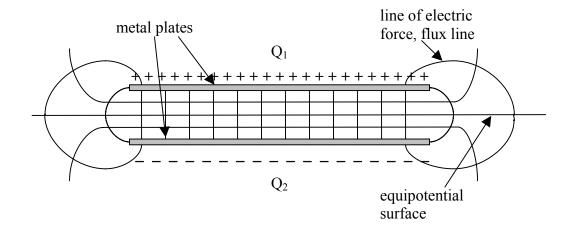
Figure 4-5. Electric field for parallel plates. (Baxter, 1997. p8)
