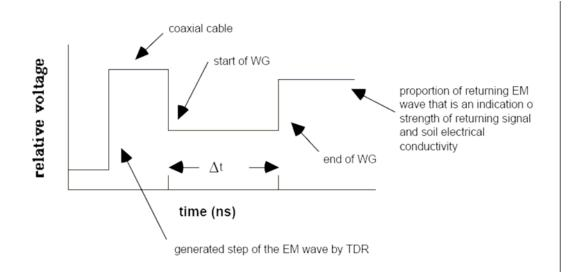
Figure 3-2. Schematic diagram of an EM wave generated by a step pulse TDR system at it travels along the coaxial cable and down the waveguides (WG) into the soil. (ICT International, 2004. p3.)
