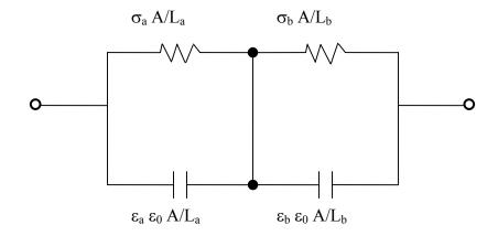
Figure 4-2. Maxwell's capacitor - equivalent circuit. (Baxter, 1997. p13)
