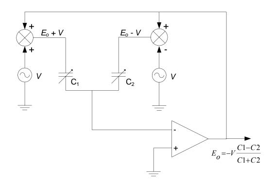
Figure 5-8. Feedback circuit
