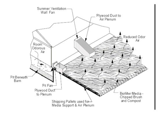
Figure 2-2. Biofilter construction. (Schmidt et al., 2004. p14)
