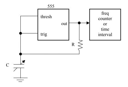
Figure 5-2. RC oscillator circuit.
