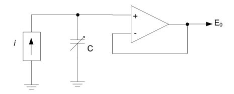
Figure 5-6. High-Z circuit.
