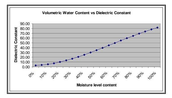
Figure 6-5. Volumetric water content vs. dielectric constant.
