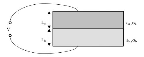
Figure 4-1. Maxwell's capacitor. (Baxter, 1997. p13)
