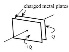
Figure 4-3. Air in the gap between the charged plates.
