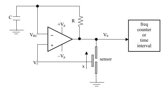
Figure 5-4. Bridge circuit with RC oscillator.
