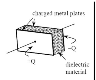
Figure 4-4. Dielectric material (insulator) between the charged plates.
