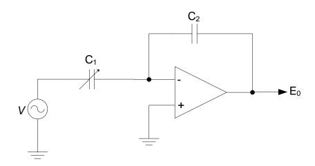
Figure 5-7. Low-Z circuit.
