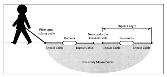
Figure 3-1. Schematic of the OhmMapper instrument. (Walker and Houser, 2002. p729.)
