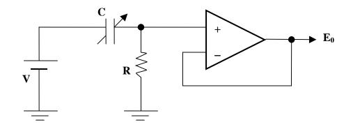
Figure 5-1. DC capacitance circuit.
