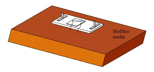
Figure 6-3. Capacitive sensor in a biofilter media.
