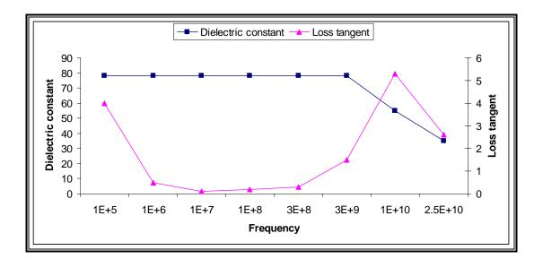
Figure 6-8. Dielectric constant and loss tangent of water vs. frequency at 25°C. (von Hippel, 1954).
