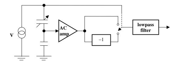
Figure 5-5. Synchronous demodulator circuit.
