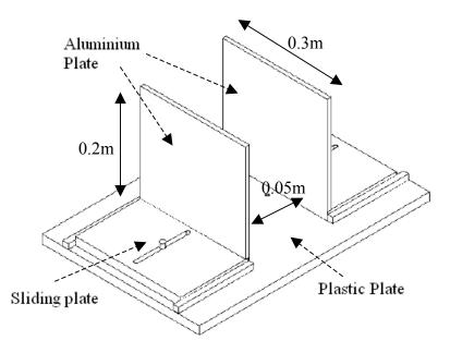
Figure 6-1. Parallel-plate setup. (Abdel et al., 2002. p4.)
