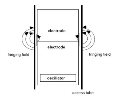
Figure 3-4. Schematic diagram of capacitance probe in an access tube (Source from White and Zegelin, 1994)
